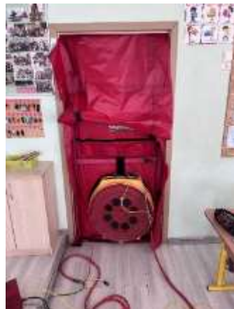
Figure 3. Blower door test.
