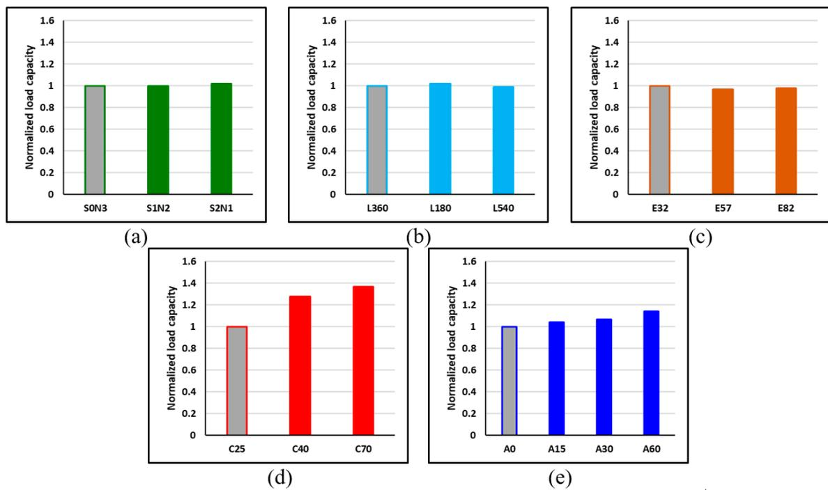
**Figure 29.** Comparisons of the effect of SMA on load capacity of the BCJ for the (a) SMA–steel reinforcement ratio, (b) lengths of SMA bars, (c) elastic modulus of SMA, (d) compressive strength of concrete, and (e) axial load level.
