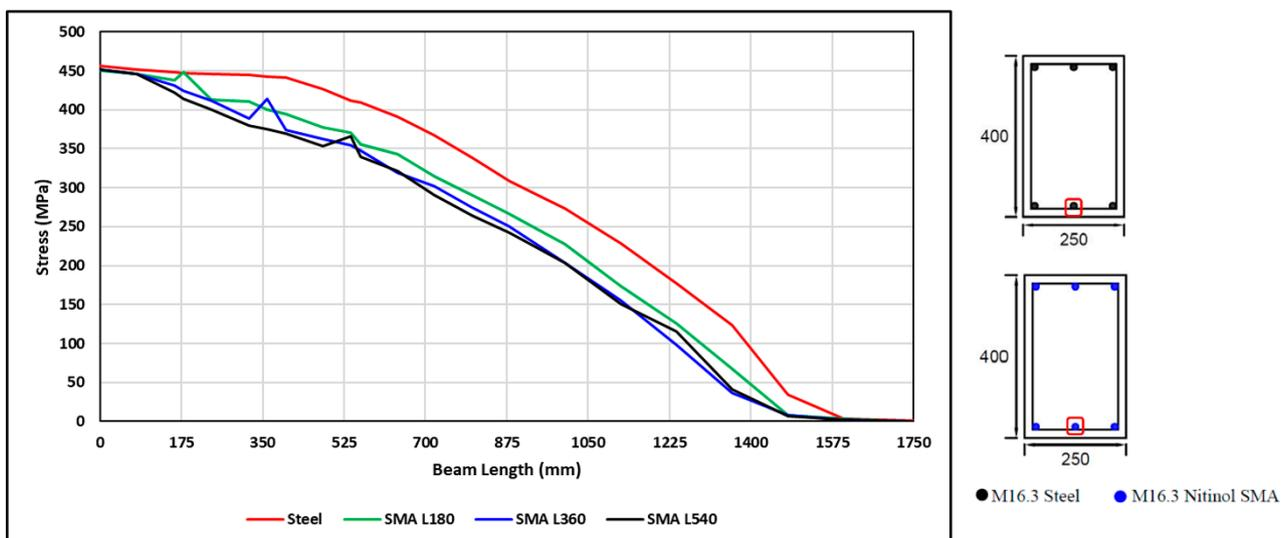
**Figure 18.** Stress of the beam reinforcement rebar using different lengths of SMA under monotonic pull loading versus the beam length at 8% drift.
