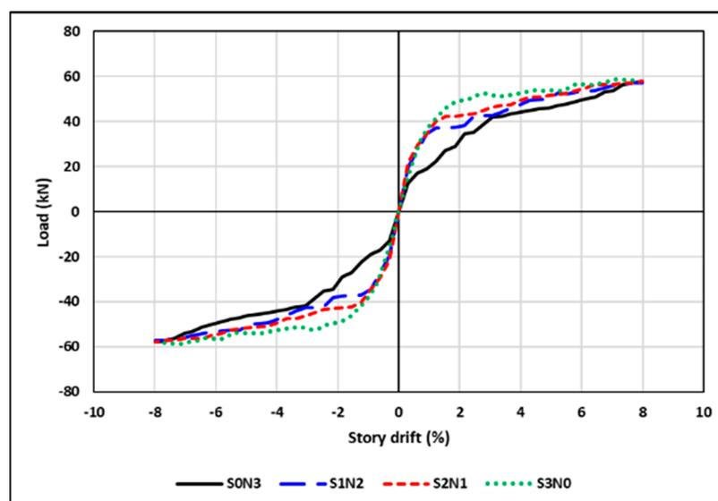
**Figure 14.** Numerical beam tip-load versus story drift envelopes of the C25-A0-S3N0, C25-A0-S1N2, C25-A0-S2N1, and C25-A0-S0N3 specimens.
