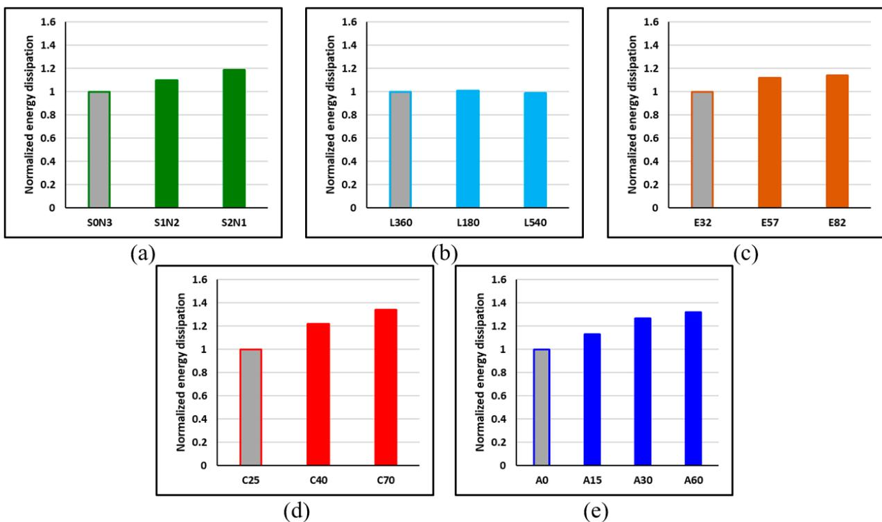
**Figure 33.** Comparisons of the effect of SMA on energy dissipation of the BCJ for the (a) SMA–steel reinforcement ratio, (b) lengths of SMA, (c) elastic modulus of SMA, (d) compressive strength of concrete, and (e) axial load level.
