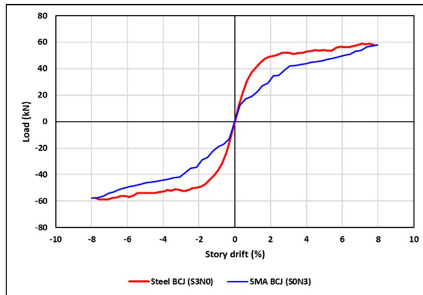
**Figure 10.** Numerical beam tip-load versus story drift envelope of the specimens C25-A0-S3N0 and C25-A0-S0N3.
