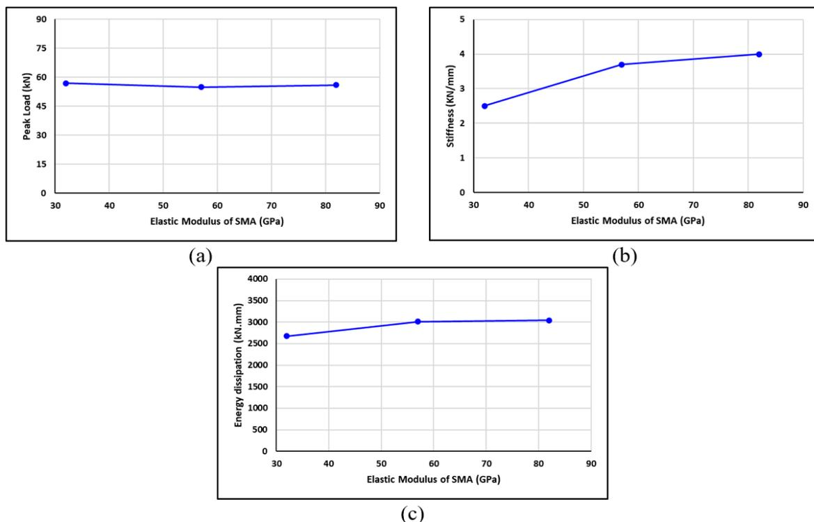
**Figure 22.** Effect of SMA elastic modulus of the BCJ on (a) load capacity, (b) stiffness, and (c) energy dissipation.
