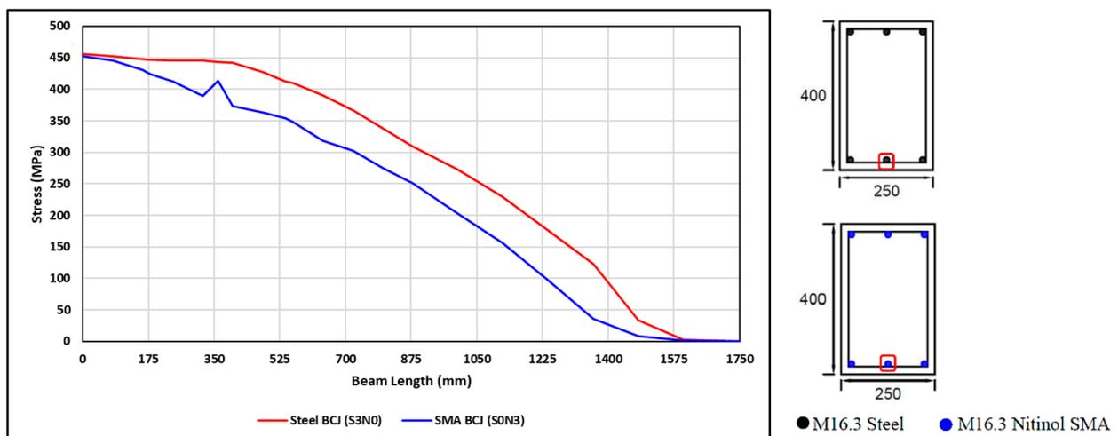
**Figure 11.** Stress of the beam reinforcement rebar under monotonic pull loading versus the span length of the beam at 8% drift.
