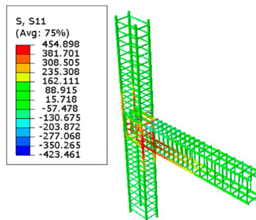
**Figure 9.** Stress in the reinforcement RC-BCJ as obtained from FE.
