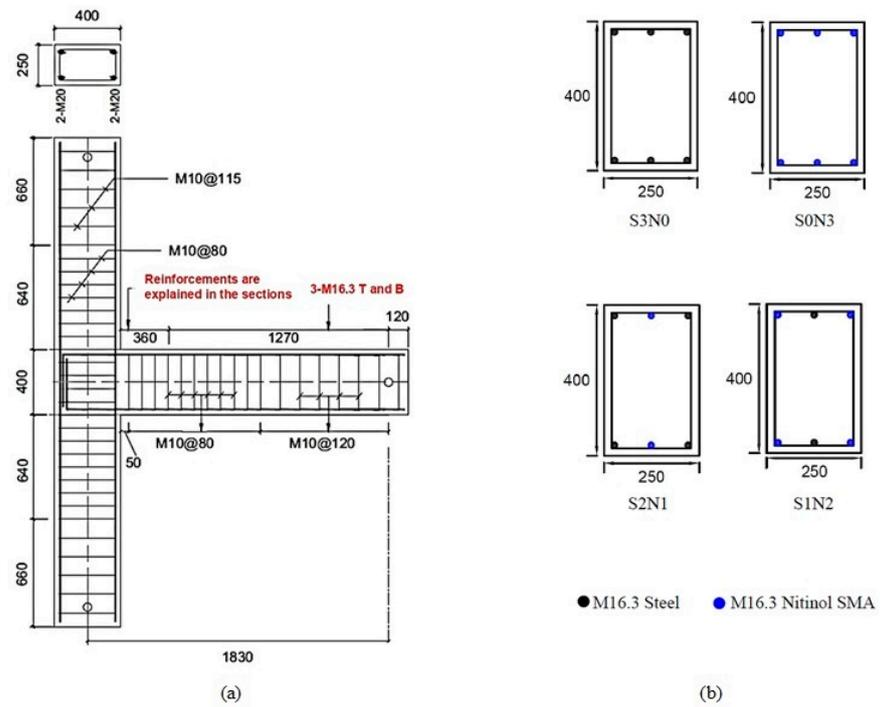
**Figure 7.** (a) Typical reinforcement details of the specimens. (b) Reinforcement details at the plastic hinge of RC-BCJ specimens (all dimensions in mm).
