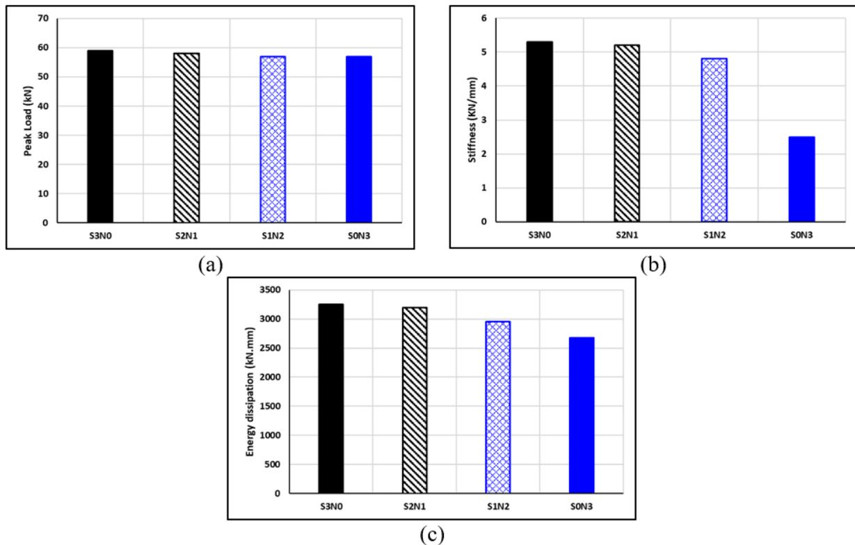
**Figure 15.** Effect of SMA-steel reinforcement ratios of the BCF on (a) load capacity, (b) stiffness, and (c) energy dissipation.
