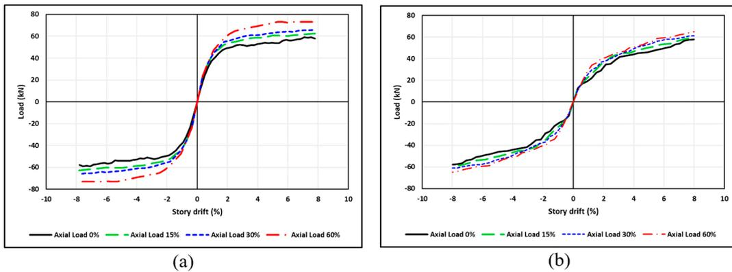
**Figure 26.** Numerical beam tip-load versus story drift envelopes of the BCJ (a) C25-A0-S3N0, C25-A15-S3N0, C25-A30-S3N0 and C25-A60-S3N0 specimens; (b) C25-A0-S0N3, C25-A15-S0N3, C25-A30-S0N3 and C25-A60-S0N3 specimens.
