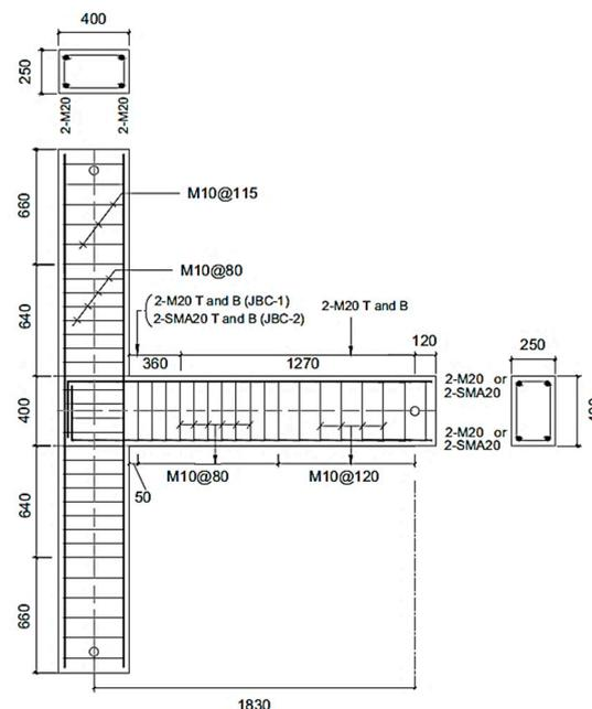
**Figure 1.** Reinforcement details of specimens, steel-BCJ and SMA-BCJ (all dimensions in mm). Reprinted from [19], with permission from Taylor and Francis.
