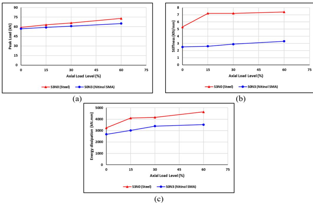
**Figure 28.** Effect of axial load level of the BCJ on (a) load capacity, (b) stiffness, and (c) energy dissipation.
