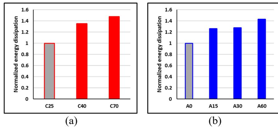
Figure 34. Comparisons of the effect of steel rebars on the energy dissipation of BCJ for: (a) concrete strength; (b) axial load level.
