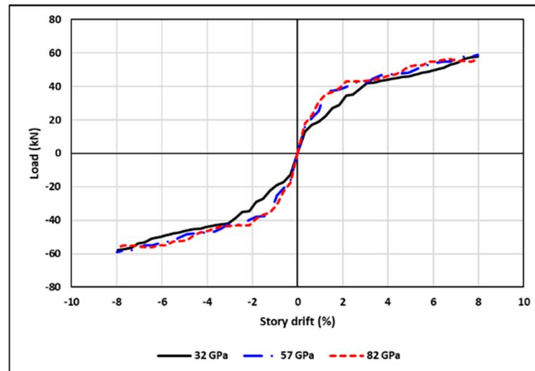
**Figure 21.** Numerical beam tip-load versus story drift envelope of the specimens C25-A0-S0N3, C25-A0-S0N3-E57 and C25-A0-S0N3-E82.
