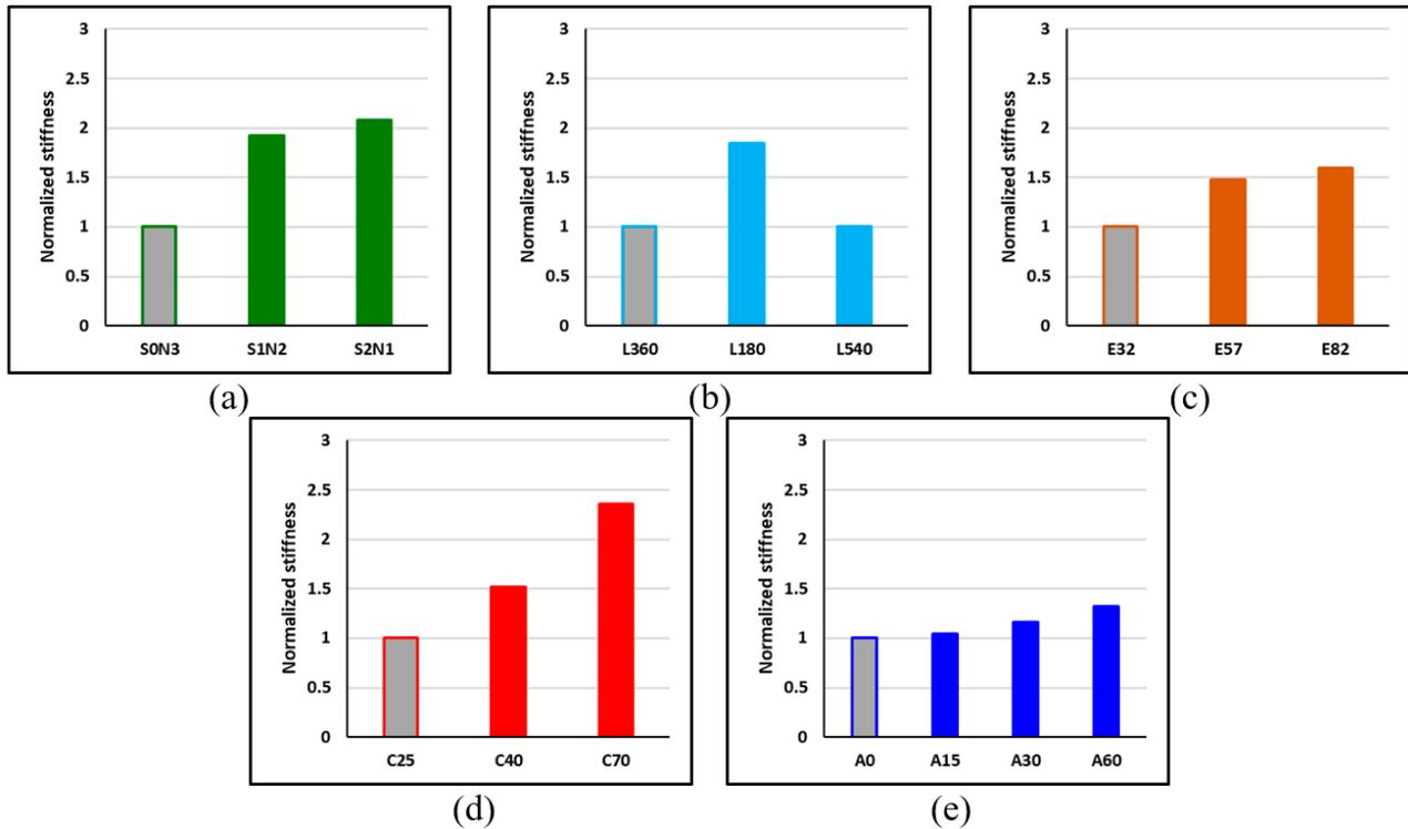
**Figure 31.** Comparisons of the effect of SMA on stiffness of the BCJ for the (a) SMA–steel reinforcement ratio, (b) lengths of SMA, (c) elastic modulus of elasticity of SMA, (d) compressive strength of concrete, and (e) axial load level.
