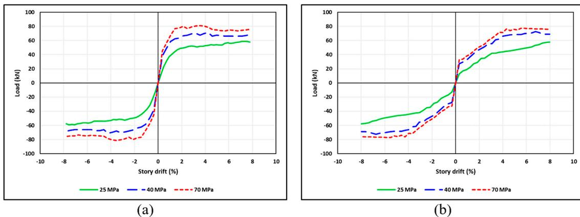
**Figure 23.** Numerical beam tip-load versus story drift envelopes of the specimens (a) C25-A0-S3N0, C40-A0-S3N0 and C70-A0-S3N0 (b) C25-A0-S0N3, C40-A0-S0N3 and C70-A0-S0N3.
