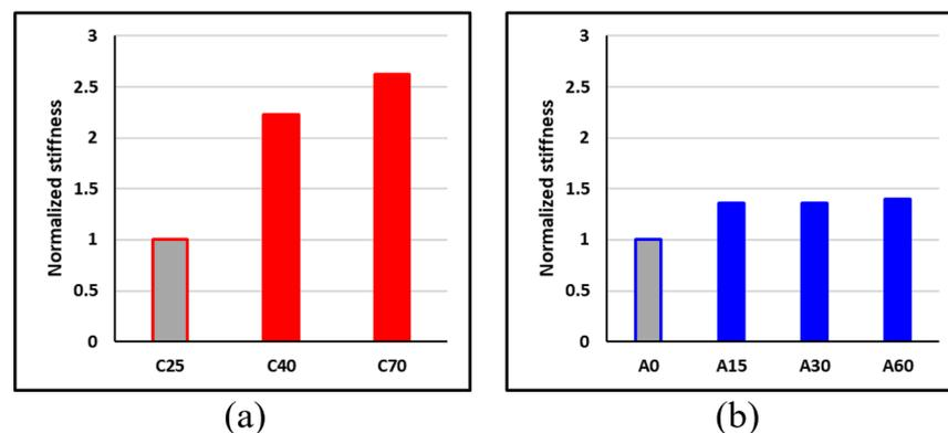
**Figure 32.** Comparisons of the effect of steel rebars on stiffness of BCJ for: (a) concrete strength; (b) axial load level.
