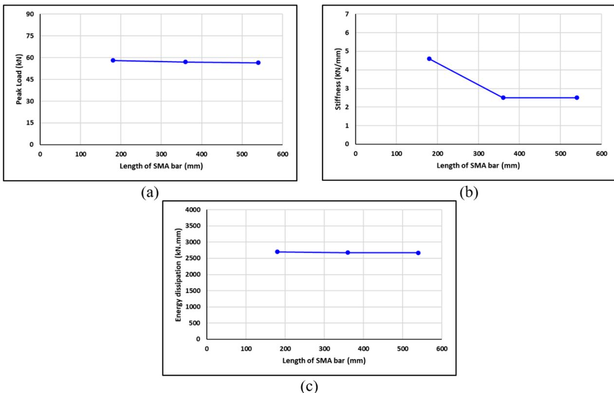
**Figure 20.** Effect of SMA bar length of the BCI on (a) load capacity, (b) stiffness, and (c) energy dissipation.
