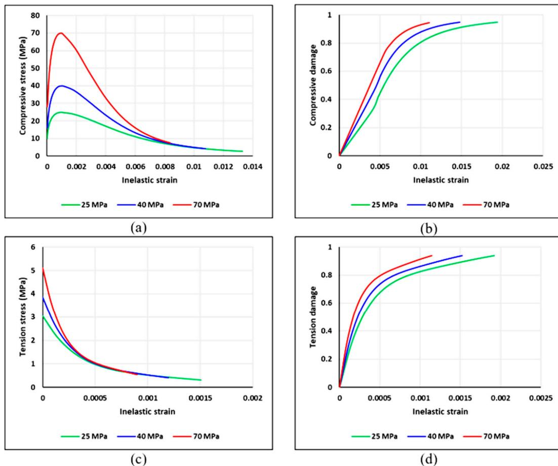
**Figure 13.** Definition of concrete damage–plasticity model parameters in ABAQUS: (a) compressive stress vs. inelastic strain, (b) compressive damage vs. inelastic strain, (c) tensile stress vs. cracking strain, and (d) tensile damage vs. cracking strain.
