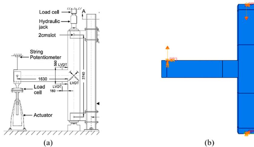
**Figure 4.** Boundary conditions of RC-BCJ: (a) experimental, reprinted from [19], with permission from Taylor and Francis. (b) Numerical.
