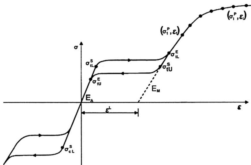
**Figure 5.** Performance of superelastic material under uniaxial tension (ABAQUS Manual). Reprinted from [21], with permission from Creative Commons Attribution (CC BY) license.
