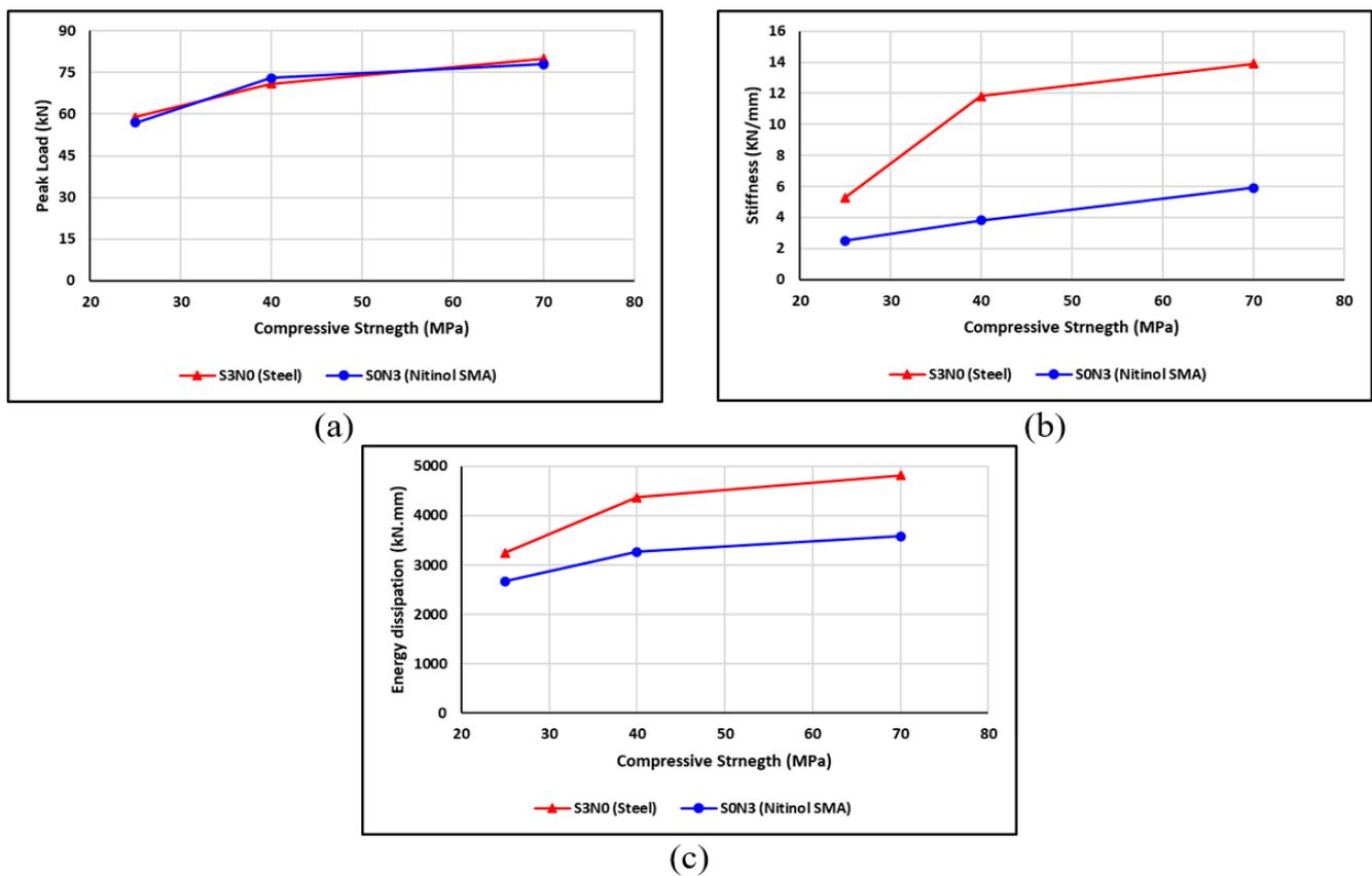
**Figure 25.** Effect of compressive strength of concrete of the BCJ on (a) load capacity, (b) stiffness, and (c) energy dissipation.
