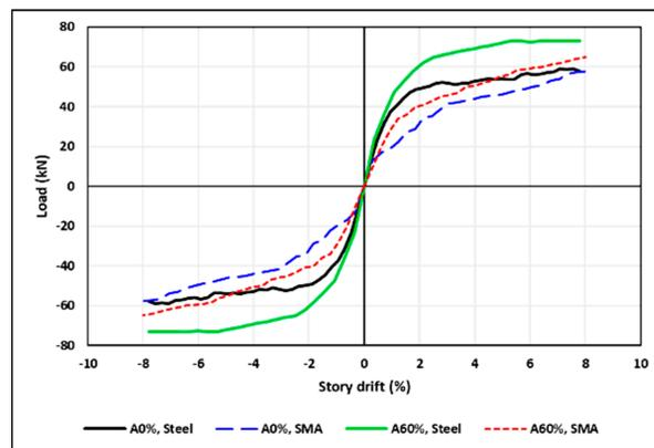
**Figure 27.** Effect of axial load level on the load capacity of the BCJ.
