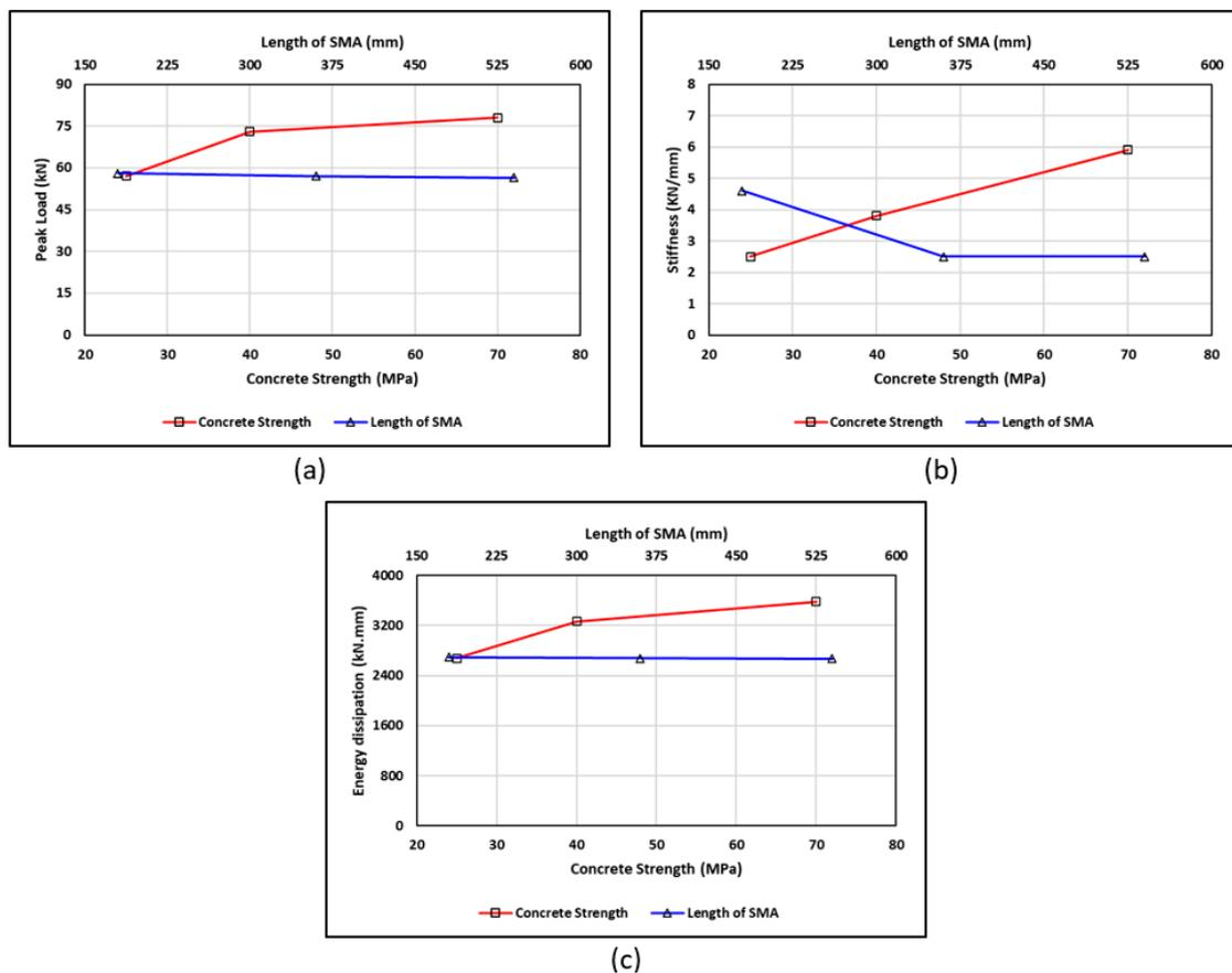
Figure 35. Comparisons of the effect of the length of SMA and concrete strength parameters on the BCJ for: (a) peak load, (b) stiffness, and (c) energy dissipation.
