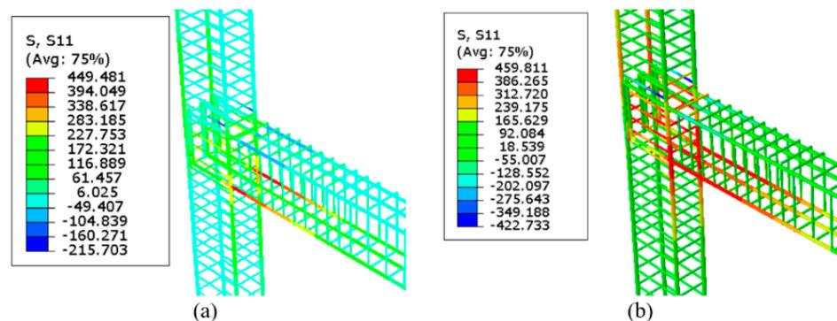
**Figure 16.** Stresses of steel and SMA rebars of S2N1 specimen during push loading at (a) 2.8% story drift and (b) 8% story drift.
