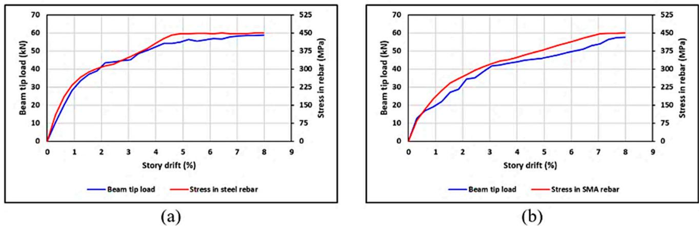
**Figure 12.** Comparisons of the numerical beam tip load and stresses in rebars versus story drift of the specimens: (a) C25-A0-S3N0 and (b) C25-A0-S0N3.
