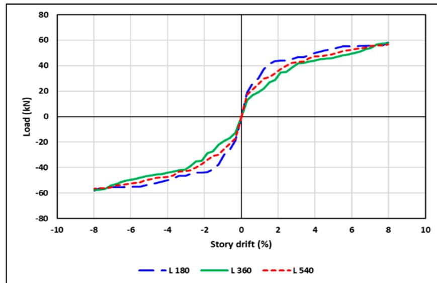
**Figure 19.** Numerical beam tip-load versus story drift envelopes of the specimens C25-A0-S0N3, C25-A0-S0N3-L180 and C25-A0-S0N3-L540.
