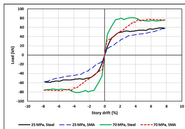
**Figure 24.** Comparison of effect of concrete strength on the behavior of BCJ between reinforced with steel and SMA.
