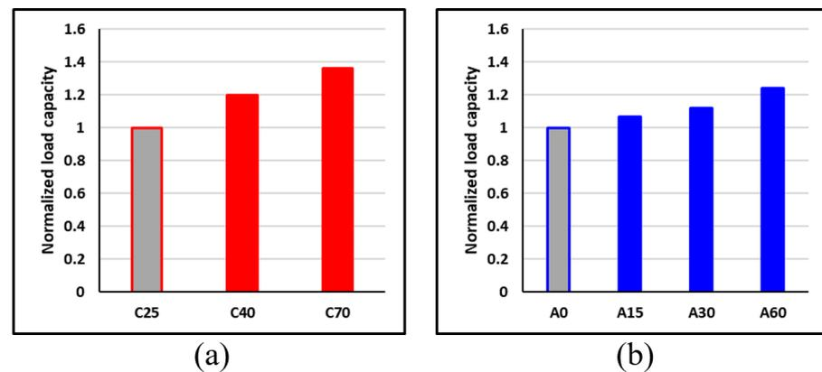
**Figure 30.** Comparisons of the effect of steel rebars on load capacity of BCJ for: (a) concrete strength; (b) axial load level.
