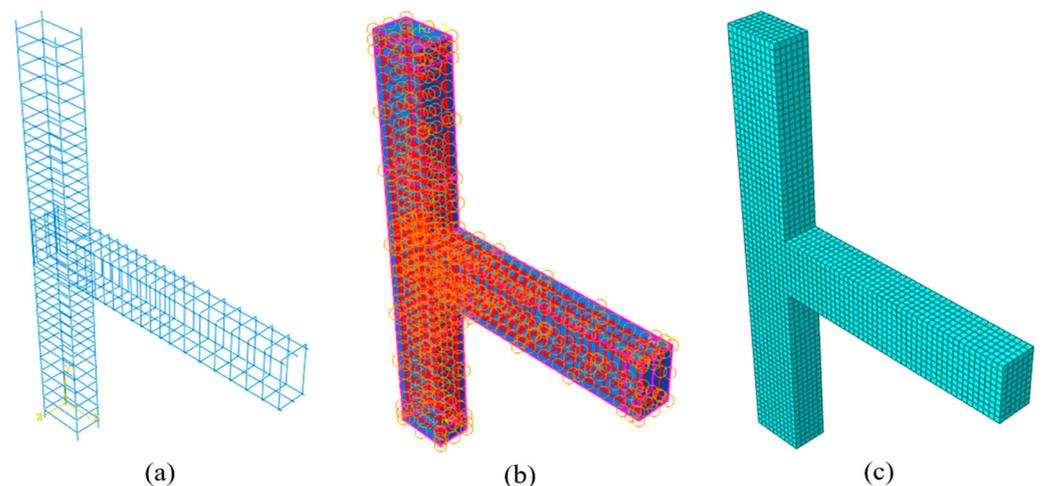
**Figure 3.** (a) Reinforcement of RC beam column joint. (b) Embedded region contact between concrete and reinforcement. (c) Typical finite element mesh of RC-BCJ.
