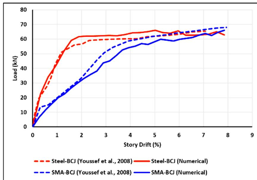
**Figure 6.** Experimental and numerical beam tip-load versus story drift envelope for the specimens steel-BCJ and SMA-BCJ [19].
