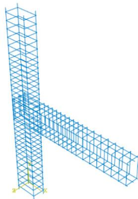
**Figure 8.** Reinforcement RC-BCJ as obtained from FE.
