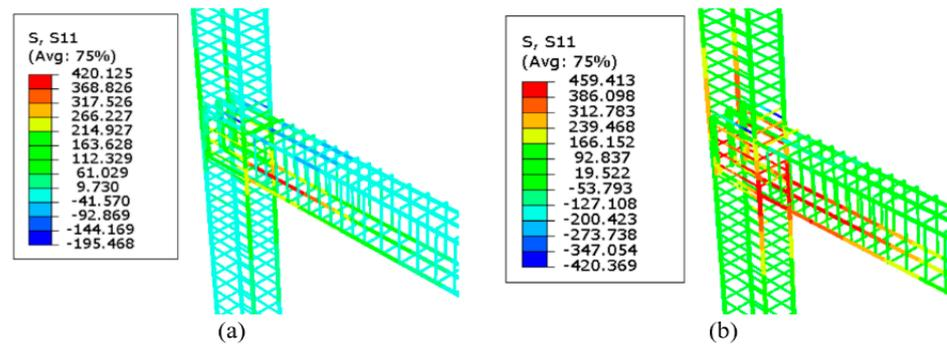
**Figure 17.** Stresses of steel and SMA rebars in S1N2 specimen during push loading at (a) 2.8% story drift and (b) 8% story drift.
