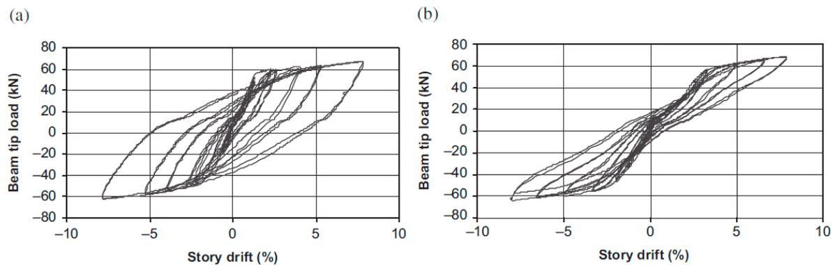
**Figure 2.** Beam tip load–story drift relationship of specimens: (a) steel-BCJ and (b) SMA-BCJ. Reprinted from [19], with permission from Taylor and Francis.
