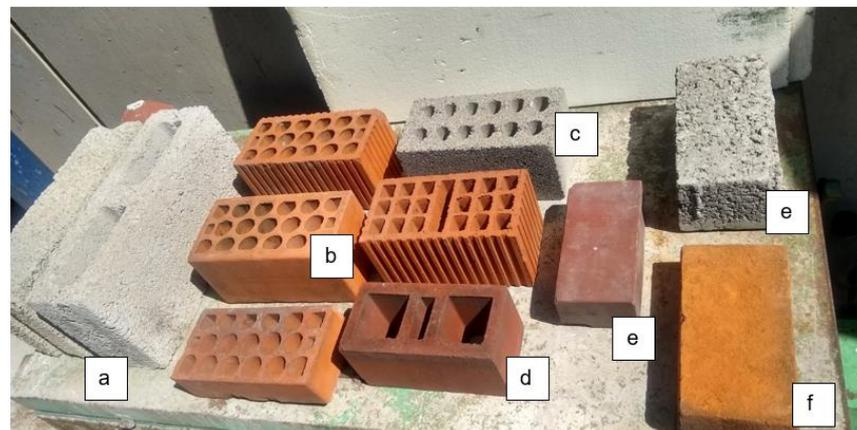
**Figure 39.** Various types of masonry units used in Mexico (Credit: L. Flores).
