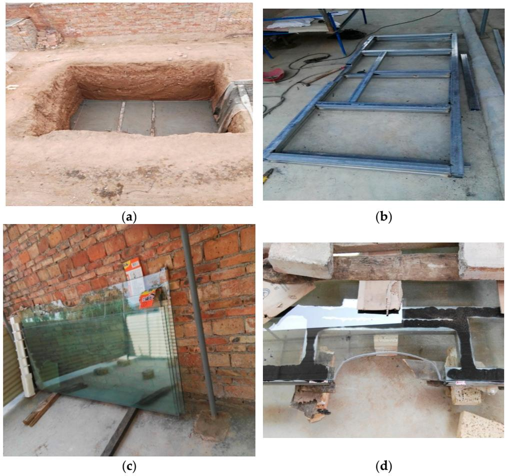
**Figure 10.** Production of model test pits. (a) Test pit; (b) Pit side support frame; (c) Tempered glass; (d) Square steel glass retaining wall.
