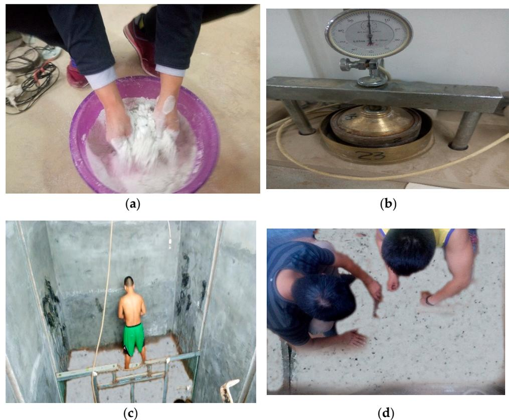
**Figure 13.** Material selection and preparation. (a) Indoor mixing; (b) Indoor wetting test; (c) Compaction process; (d) Sampling with a ring knife.
