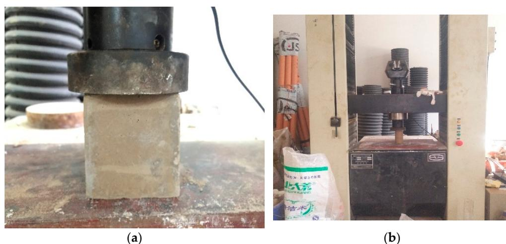
**Figure 16.** Lining material test. (a) Compressive strength test; (b) Elastic modulus test.
