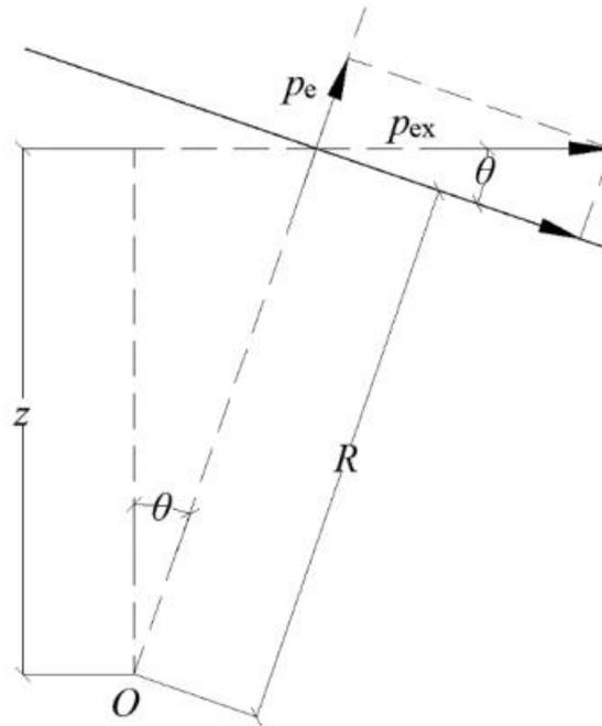
**Figure 5.** Schematic diagram of liquid inertia additional pressure on the tank wall.
