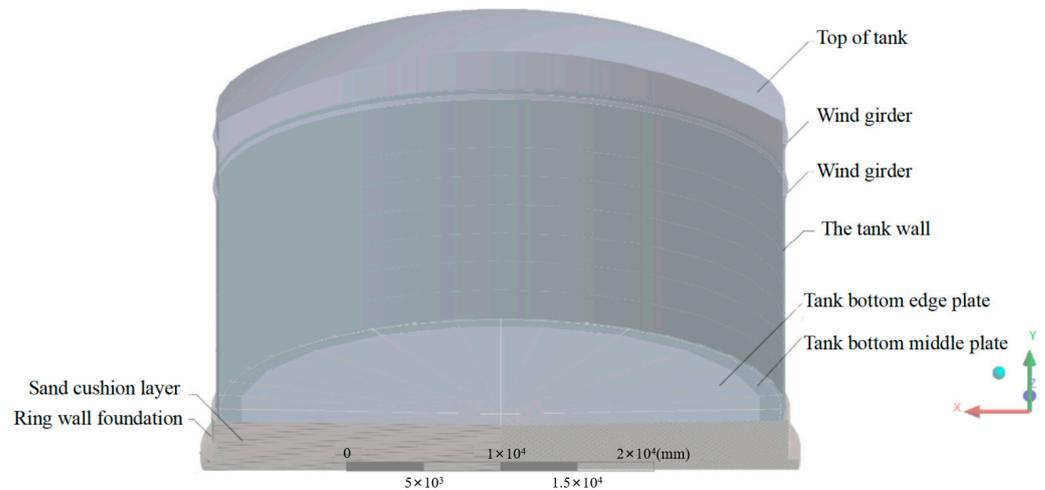
**Figure 2.** Vertical section of the model.
