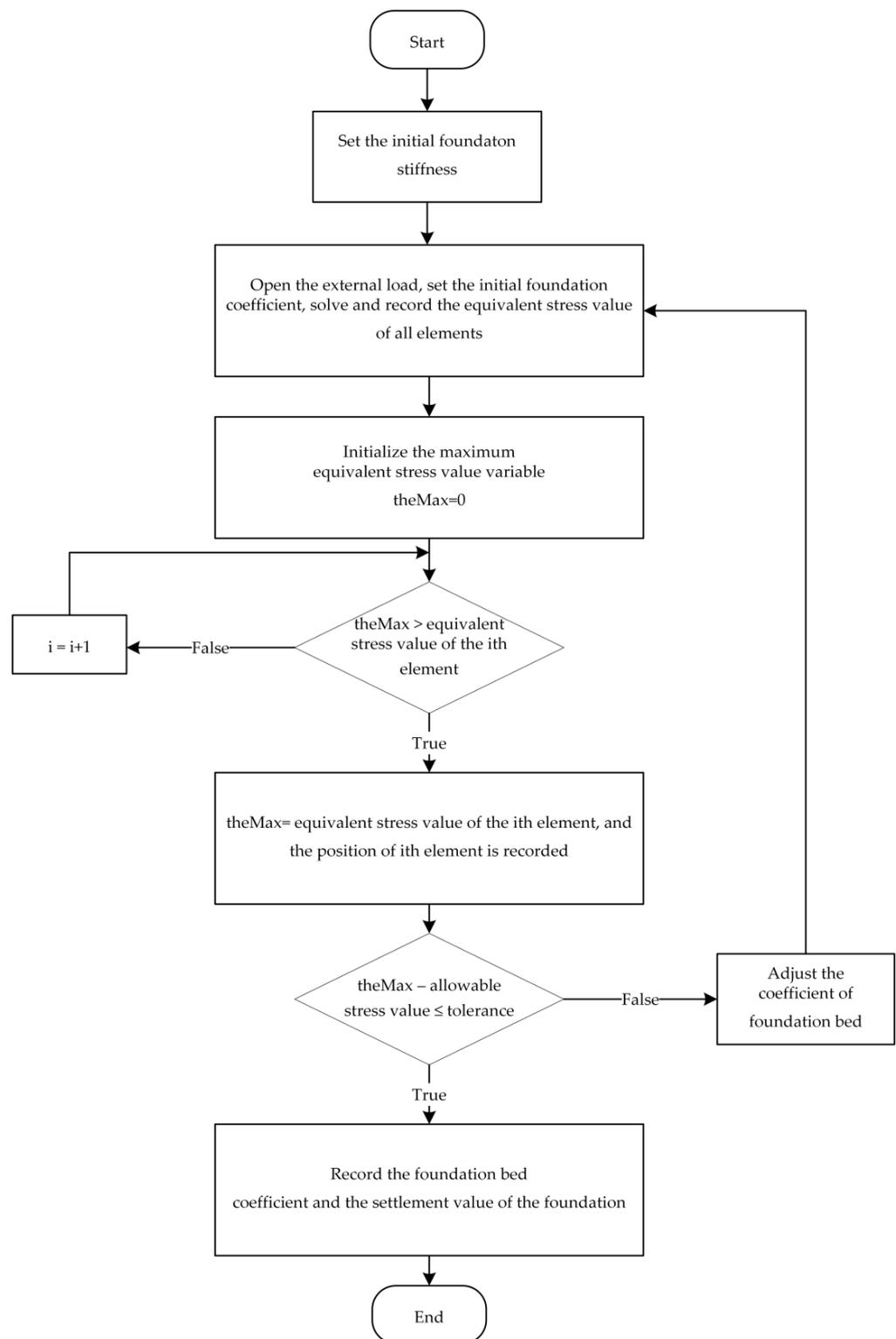
**Figure 8.** Algorithm for finding critical state of bottom stress under uneven foundation.
