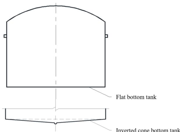
**Figure 1.** Forms of vertical tank bottoms.
