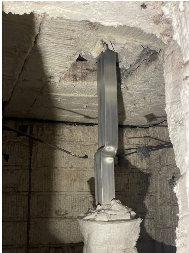
Figure 23. The aluminium column No. 2.4.3 after heat exposure.
