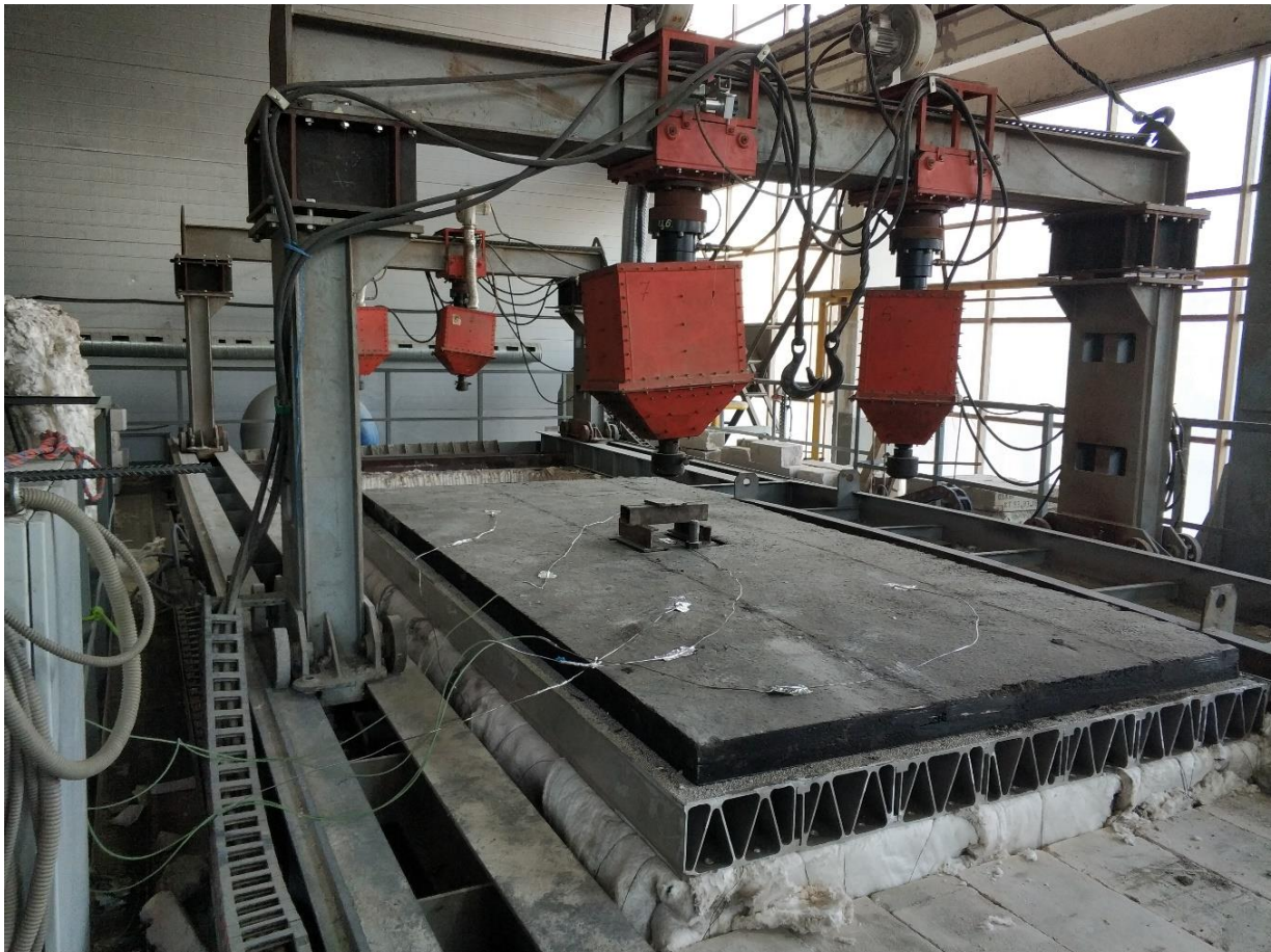
Figure 17. The aluminium orthotropic deck before testing.
