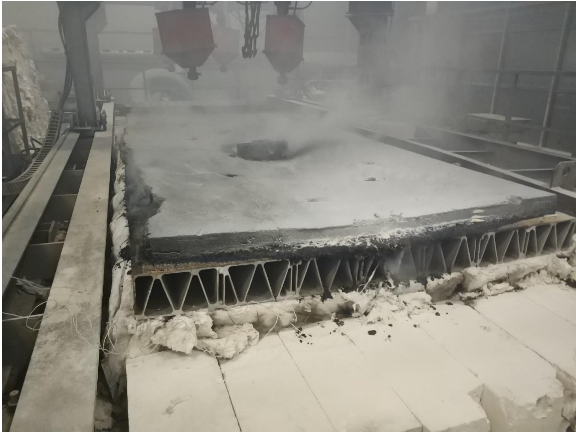
Figure 21. The aluminium orthotropic deck after testing.
