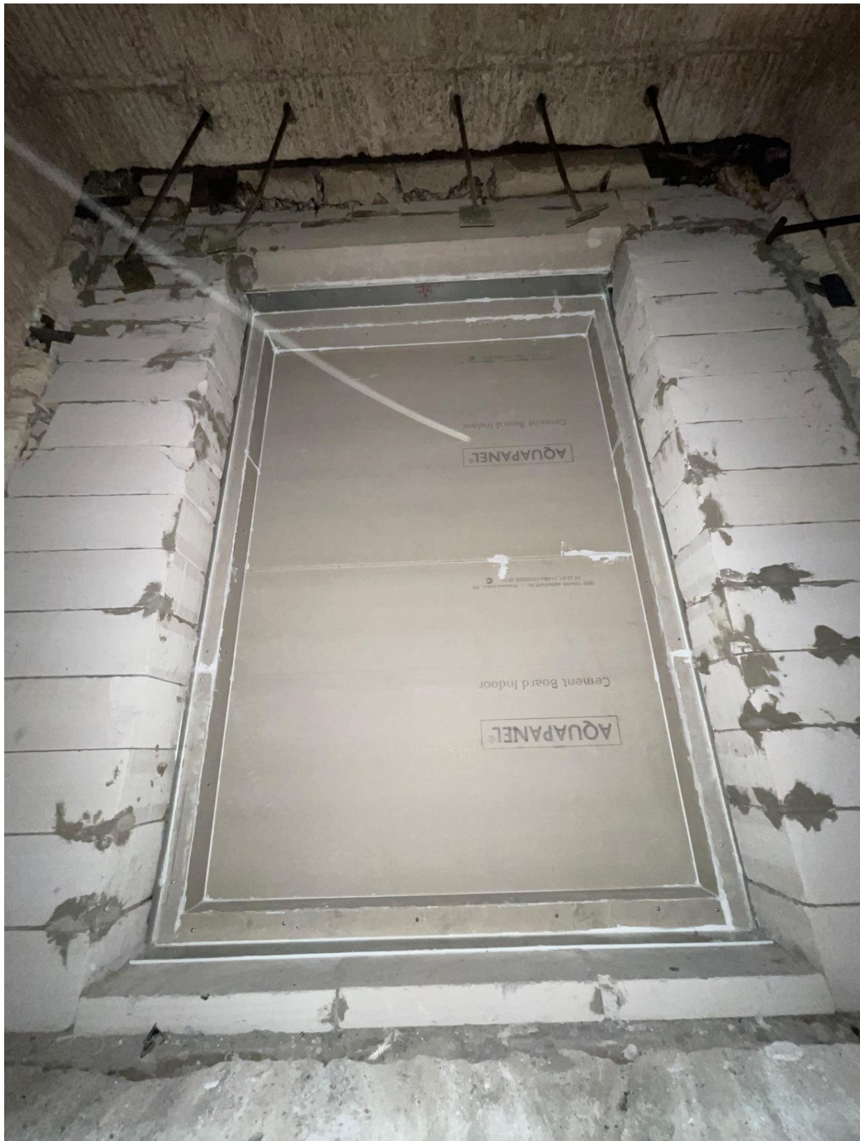
Figure 13. The attachment unit of the mullion and transom system covered with a fire-resistant cement slab before testing.
