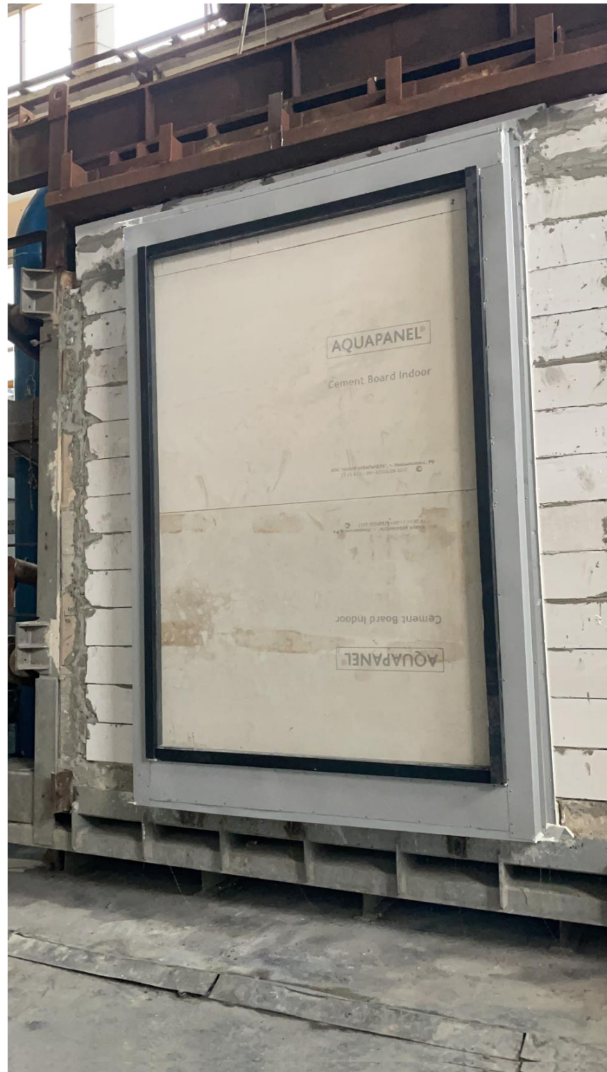
Figure 8. The unheated side of the attachment unit of the mullion and transom system before testing.
