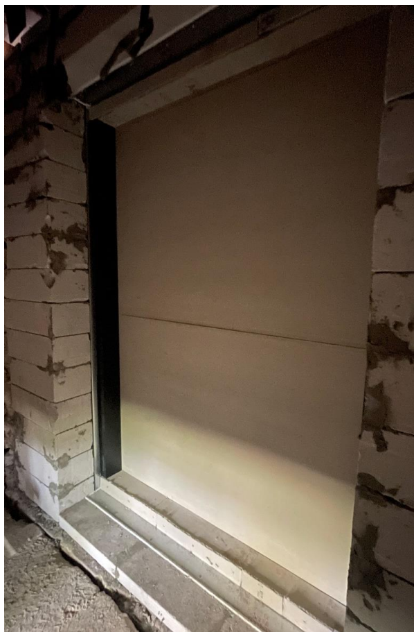
Figure 9. The heated side of the attachment unit of the mullion and transom system with a protective non-inflammable heat-insulating membrane before testing.
