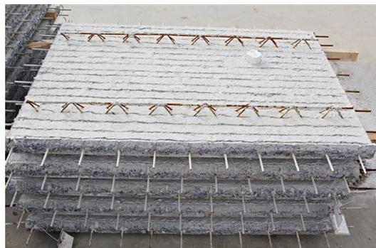
**Figure 2.** Precast concrete slab with steel truss bars.
