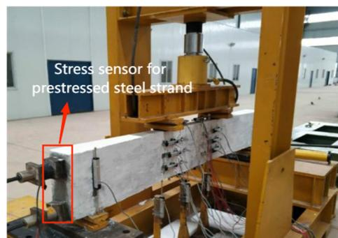
**Figure 2.** Setup of beam test: (a) schematic (units: mm); and (b) photograph.
