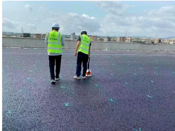
**Figure 9.** Compaction uniformity inspection.
