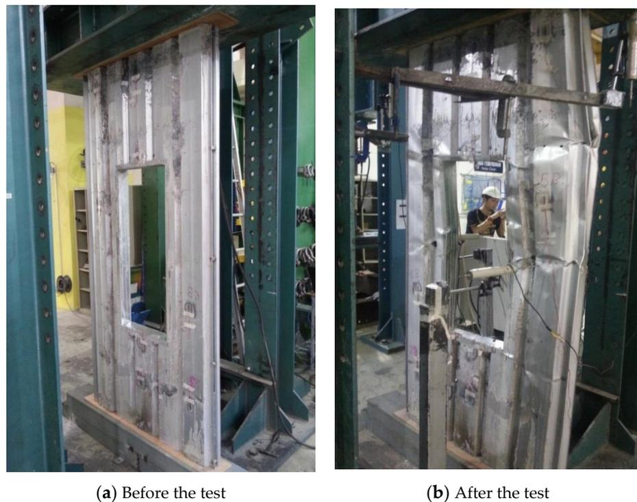
Figure 8. Failure mode of the DSPCW specimen with an opening (Ope-Oct).
