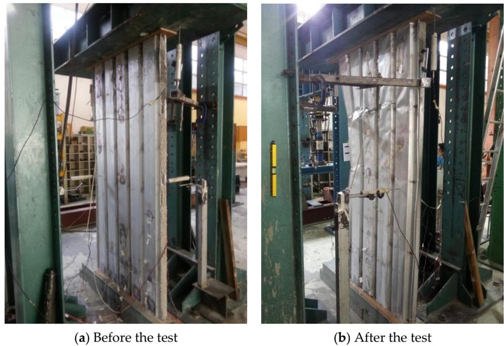
Figure 7. Failure mode of the DSPCW specimen (Oct).
