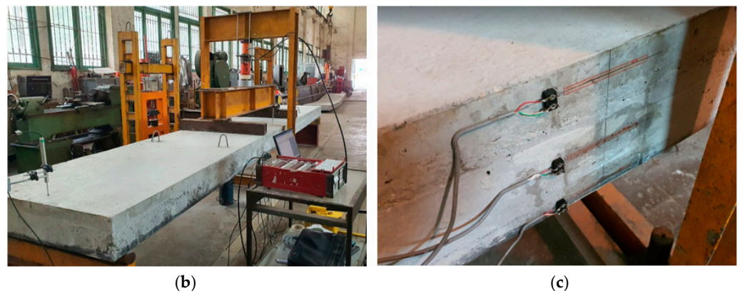
Figure 4. The testing arrangement and measuring equipment installation: (a) schema of testing arrangement; (b) testing arrangement; (c) strain gauges installation.
