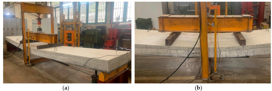
Figure 5. (a) Failure mode and (b) crack distribution of specimen M1.
