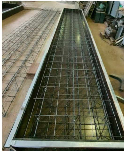
Figure 1. Dimensions (in mm) and reinforcement details of the test specimens: (a) dimensions of the test specimens; (b) cross section of specimens and reinforcement details; (c) longitudinal section of specimens and reinforcement details; (d) installation of reinforcements.
