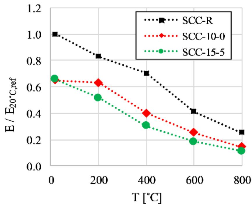
**Figure 10.** Normalised values of the modulus of elasticity ( $E$ ) concerning the value of the modulus of elasticity of the reference SCC mixture at  $T = 20^{\circ}C$ .
