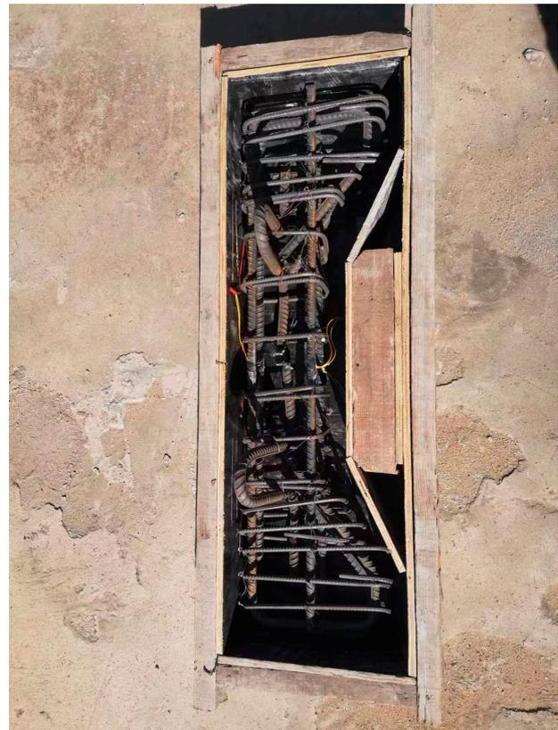
Figure 2. Preparation of specimen: (a) Design of reinforcement (units: mm), (b) Steel bar cage.
