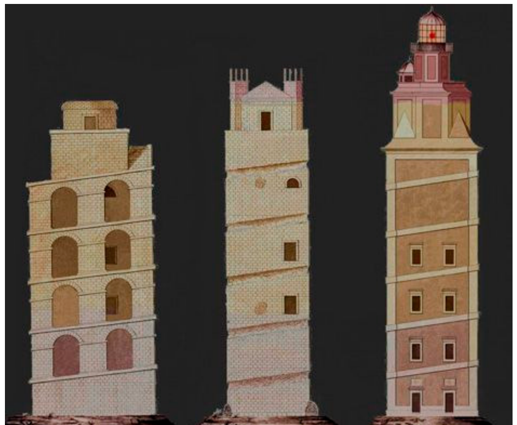
Figure 2. External appearance of the tower throughout its history, ordered chronologically from left to right: Roman period (assumed elevation, left ), late 17th century ( center ), and after the intervention carried out in the 18th century ( right ) [29].
