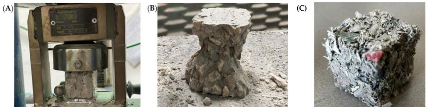
**Figure 10.**  $40 \times 40 \times 40$  mm concrete sample during (A) and after (B) compression test,  $40 \times 40 \times 40$  mm concrete sample with 100% of plastic aggregates (Plastic\_100%) after curing (C).
