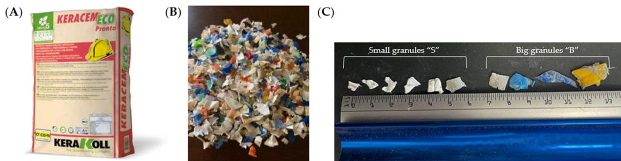
**Figure 2.** Lightweight screed components: Keracem Eco Pronto produced by Kerakoll company (A), mixed plastic granules (B), and the sizes of big “B” and small “S” plastic granules (C) derived from the recycling process.
