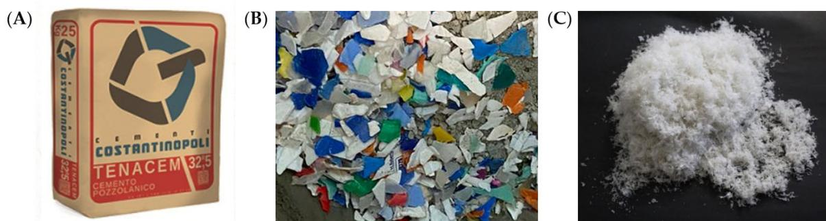
**Figure 3.** Lightweight concrete components: pozzolanic cement Tenacem 32.5 manufactured by the Cementi Costantinopoli company (A), plastic granules (B), and pulverized plastic (C).
