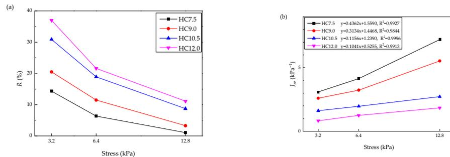
**Figure 6.** MSCR test of the HCPMA at different stress. (a)  $R$ ; (b)  $J_{nr}$ - $\sigma$  curves and linear fitting with correlation coefficient.
