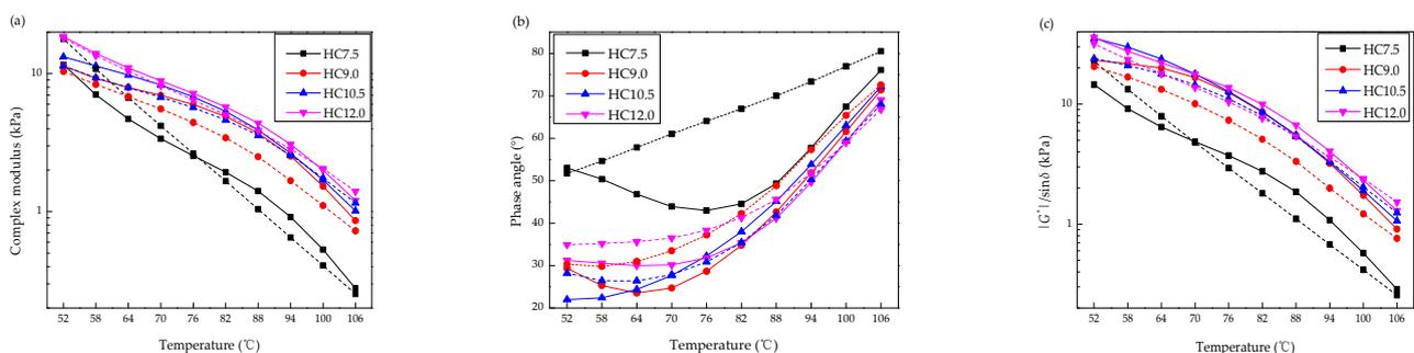
**Figure 3.** Oscillation temperature sweep of the HCPMA. (a) Complex modulus; (b) phase angle; (c) rutting parameter with solid lines for original samples, and dash lines for RTFOT residues.
