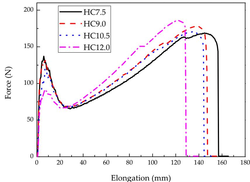
**Figure 1.** Force-elongation curves of the toughness test of HCPMA.
