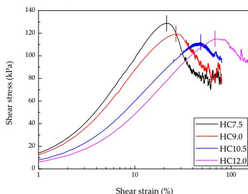
**Figure 8.** Stress–strain curves of HCPMA by amplitude sweep.
