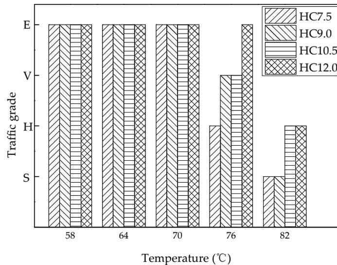
**Figure 5.** The traffic grade of various HCPMA at different temperatures.
