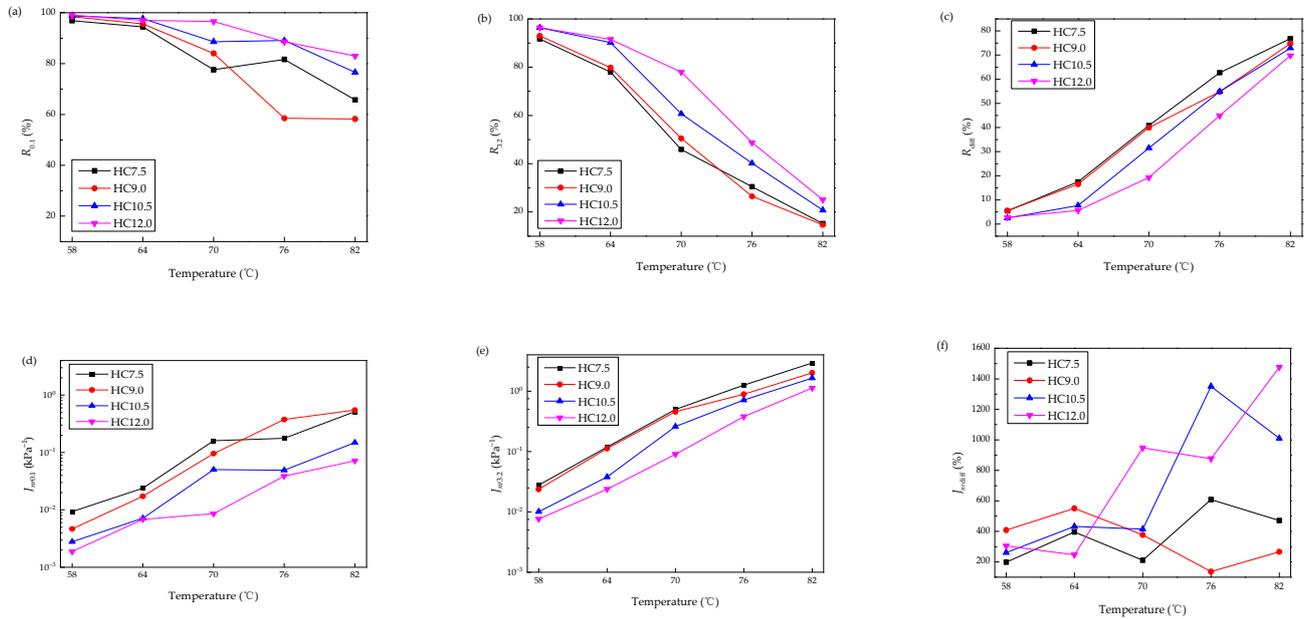
**Figure 4.** MSCR test of the HCPMA at different temperatures. (a)  $R_{0.1}$ ; (b)  $R_{3.2}$ ; (c)  $R_{diff}$ ; (d)  $J_{nr0.1}$ ; (e)  $J_{nr3.2}$ ; (f)  $J_{nr\text{diff}}$ .
