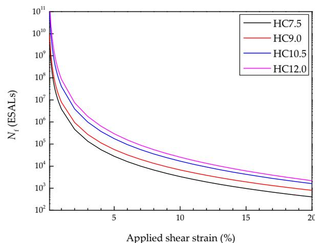
**Figure 10.**  $N_f$ -shear strain curves of HCPMA with different SBS content.
