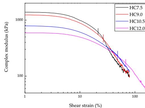
**Figure 9.** Complex modulus-strain curves of HCPMA by amplitude sweep.
