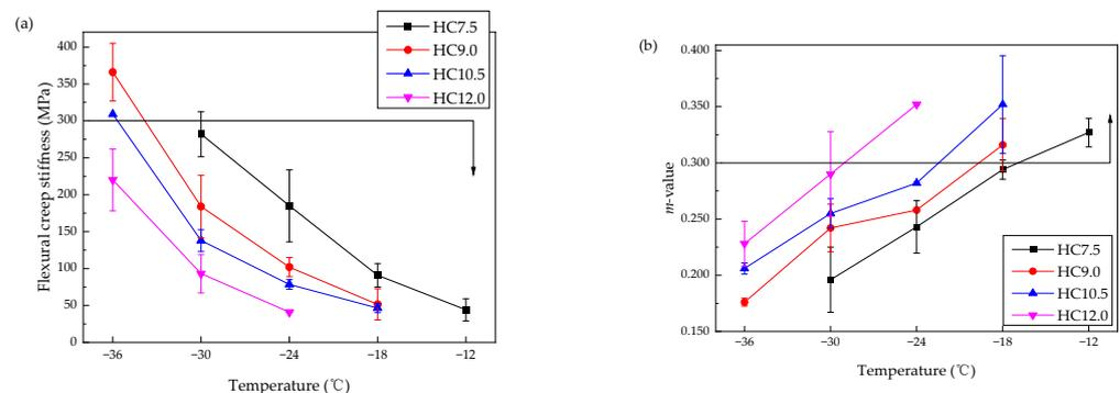
**Figure 7.** BBR results of various HCPMA at different temperatures. (a) Flexural creep stiffness; (b) creep rate.
