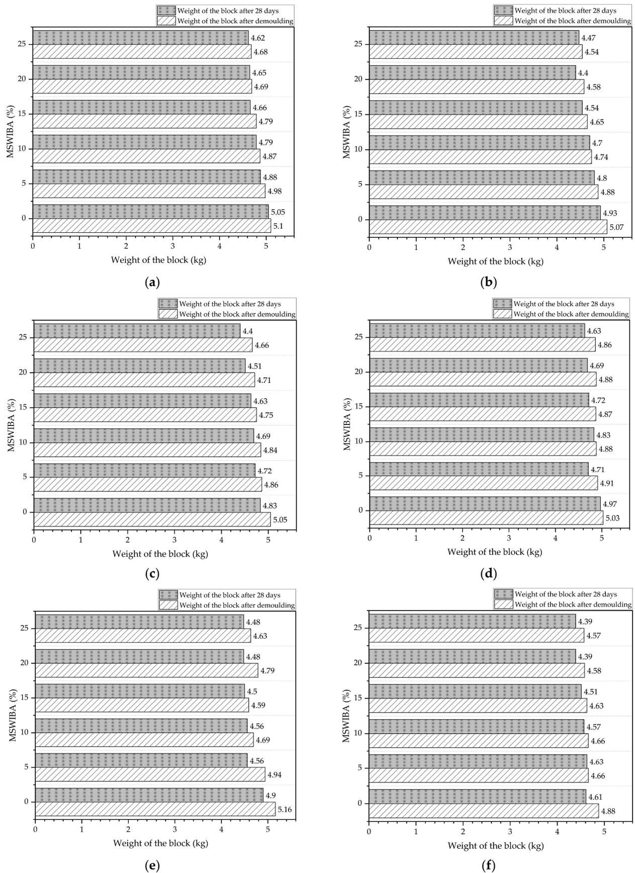
**Figure 6.** Weight of block with various % of cement content (a) 0% cement, (b) 6% cement, (c) 7% cement, (d) 8% cement, (e) 9% cement, (f) 10% cement.
