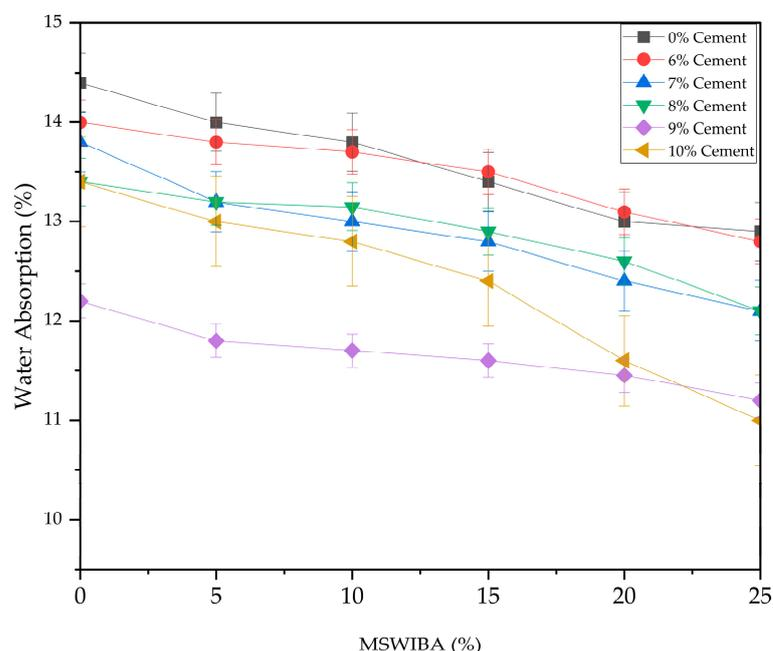
**Figure 10.** Effect of MSWIBA on the water absorption.
