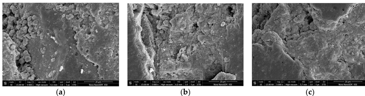
**Figure 14.** SEM analysis, (a) 10% of cement with 15% of MSWIBA, (b) 10% of cement with 25% of MSWIBA, (c) 10% of cement with 20% of MSWIBA.
