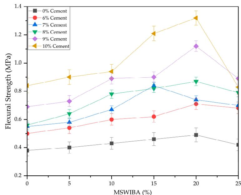
Figure 9. Effect of MSWIBA on the flexural strength.
