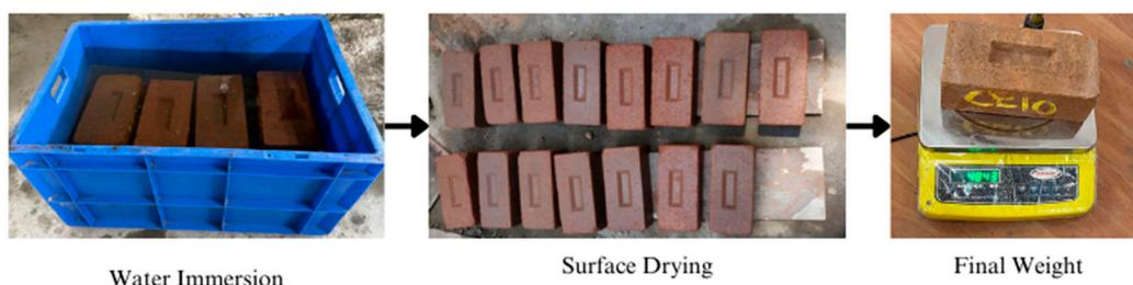
**Figure 4.** Flowchart of water absorption test.
