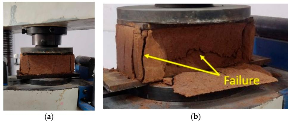
**Figure 2.** (a) Test set up for compressive strength and (b) observed crack pattern of the sample.
