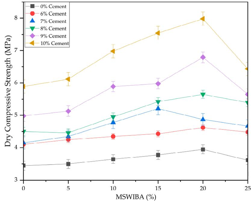
Figure 11. Dry compression strength of CSEB after alternate wetting and drying.
