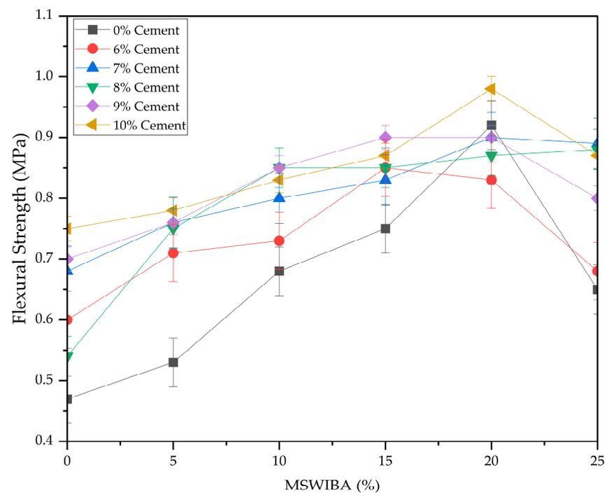
Figure 12. Flexural strength of CSEB after alternate wetting and drying.
