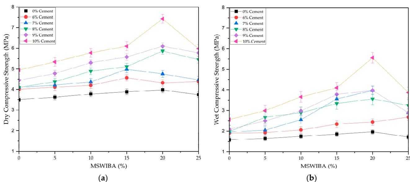
**Figure 7.** (a) Dry compression strength and (b) wet compression strength varies with MSWIBA concentration.
