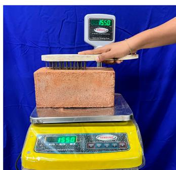
**Figure 5.** Measurement of pressure applied by wire scratch brush on the specimen.
