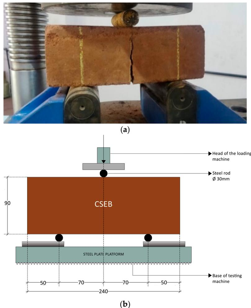
**Figure 3.** (a,b) Flexural test setup for CSEB.
