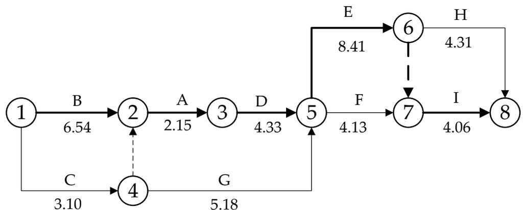
Figure 5. Adjusted network schedule considering multi-resource constraints.
