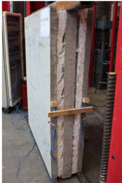
Figure 19. A failure showing substantial deformation in the foam prior to loss of bond.
