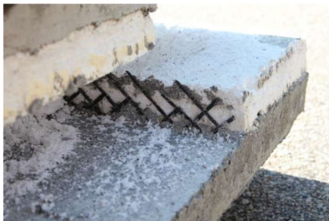
Figure 21. View of ruptured and pulled-out grid.
