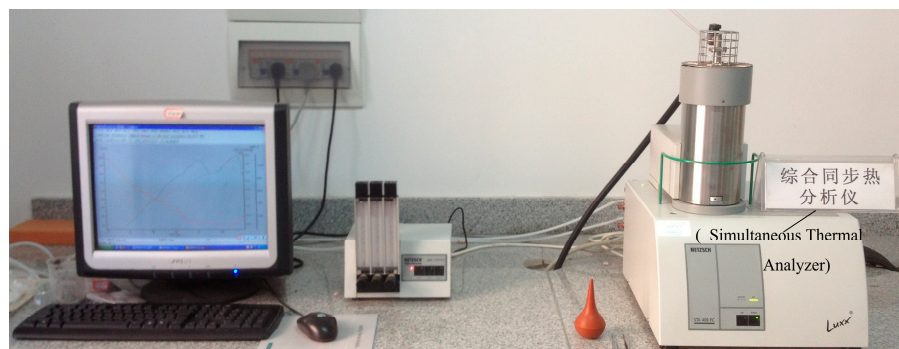
Figure 6. Thermogravimetric analysis process.
