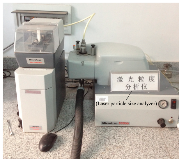
Figure 2. Laser particle size analysis.
