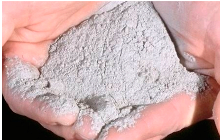
Figure 1. Carbonated recycled concrete fine.
