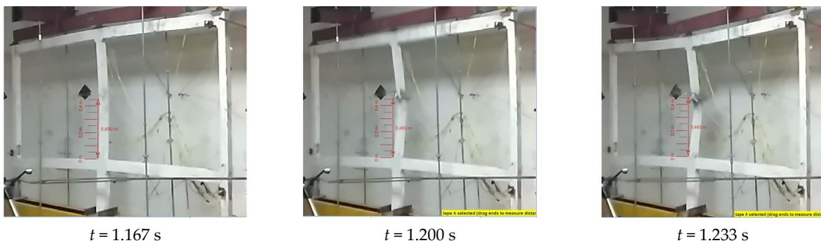
**Figure 11.** Video processing data for deformation and failure of the test frame under the corner column removal scenario.
