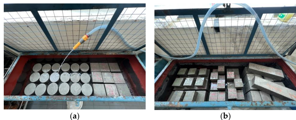
Figure 3. Preparation of samples: (a) cylinders and (b) cubes and beams.
