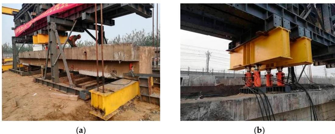
**Figure 7.** Field test. (a) Installation of the test beam; (b) loading with jacks.
