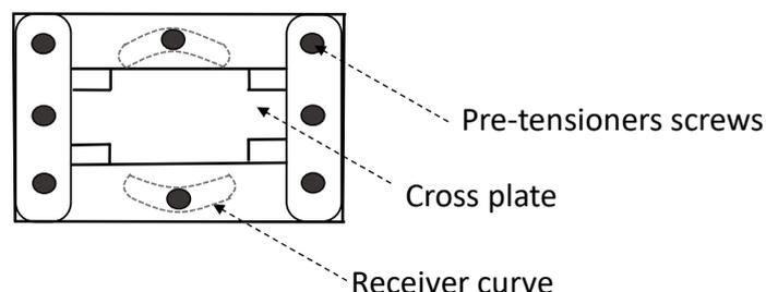
Figure 3. Pall friction damper.
