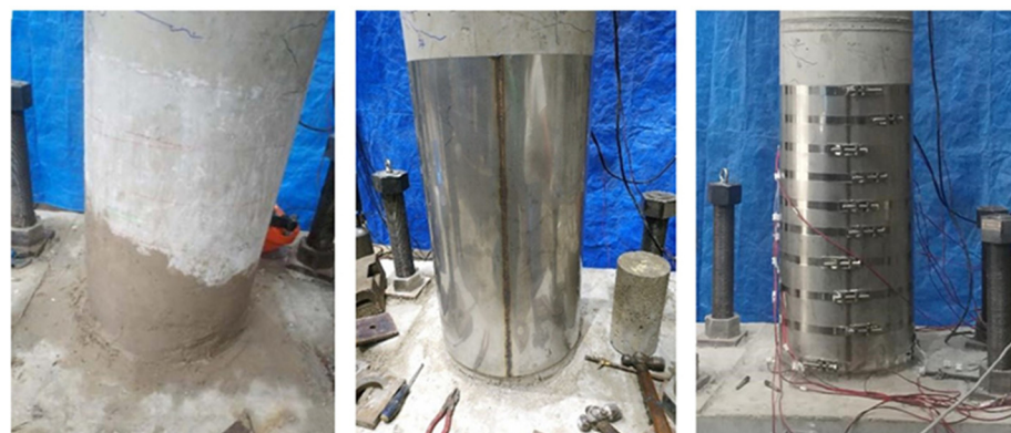
Figure 15. Steel jacketing strengthening process. Adapted from [144].
