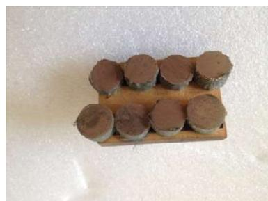
**Figure 4.** SEM sample preparation.
