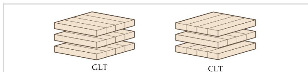
**Figure 1.** Bond directions in mass timber products, GLT and CLT [28].
