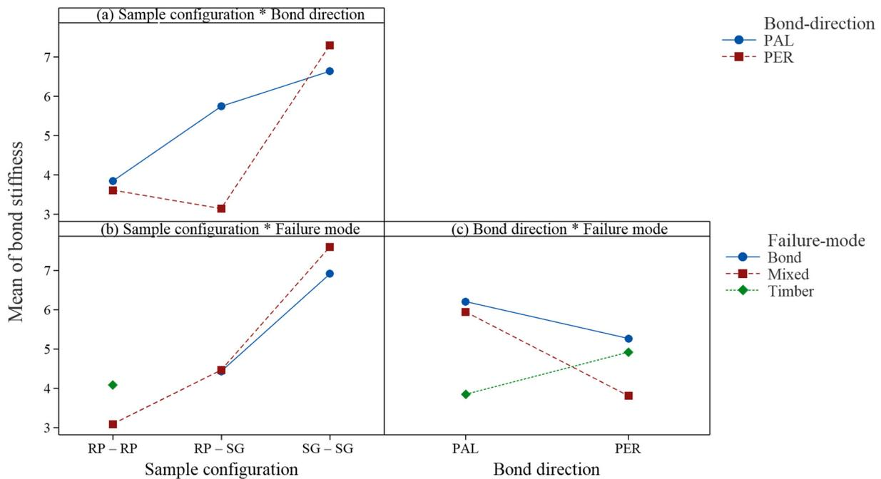
**Figure 11.** Interaction plot between sample configuration, bond direction and failure mode on bond stiffness.
