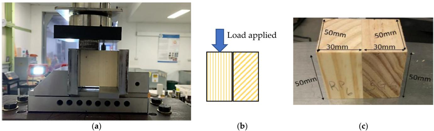
**Figure 3.** (a) Test setup, (b) direction of applied load, (c) shear plane for PER configuration.
