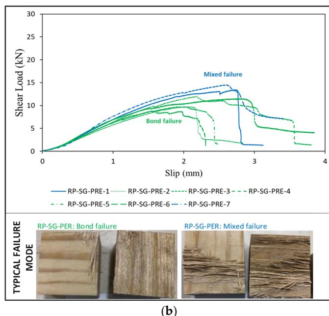
**Figure 6.** Loading curves and typical modes for RP-SG samples. (a) RP-SG-PAL, (b) RP-SG-PER.
