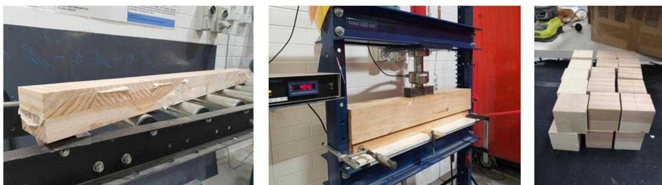
**Figure 2.** Lamellae preparation, clamping process and final specimens for testing.
