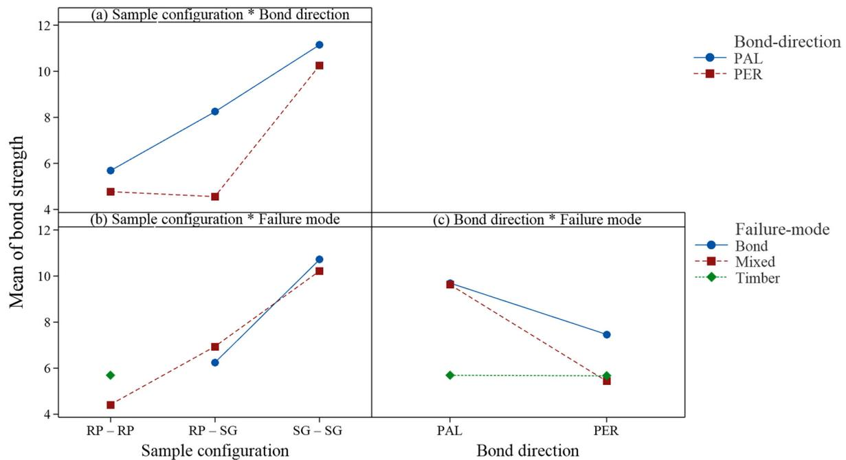
**Figure 10.** Interaction plot between sample configuration, bond direction and failure mode on bond strength.
