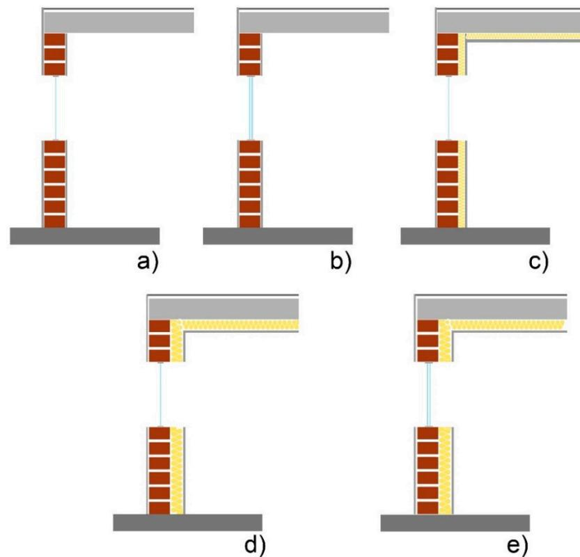
**Figure 5.** Section drawings of the different building fabric typologies used in the dynamic simulations. Each cross-section is explained below identified by its letter: (a) as built; (b) double glazing, no insulation; (c) single glazing and 3 cm of insulation (as established by the NOM-ENER-020); (d) single glazing and 5 cm of insulation (standard practice); (e) double glazing and 5 cm of insulation.
