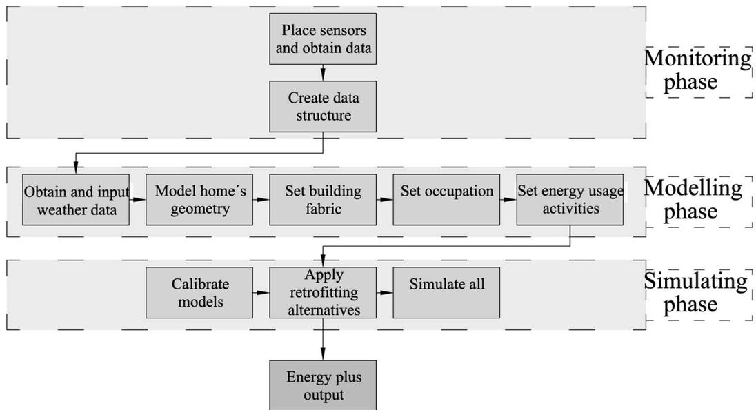
**Figure 4.** Stages of the simulation process. Stage 1 (monitoring phase) consisted of obtaining the sensors, ensuring their correct operation, and placement in the different houses. Stage 2 (modelling phase) surveyed the homes (measuring the perimeters and taking photographs). Later, these data were used in D.B. to create the simulation models. Finally, Stage 3 (simulation stage) consisted of simulations with the different building envelopes.
