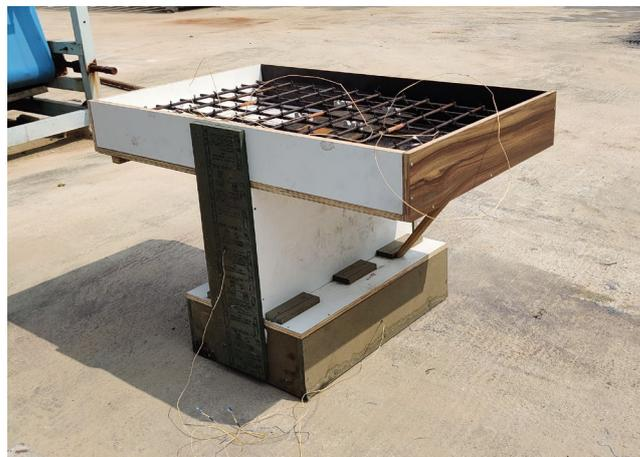
**Figure 3.** The scale-down experimental model of I-girder segment Formwork and temperature sensors spaced around the top flange.
