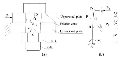
**Figure 2.** Mechanical model and mechanism diagram of bolt: (**a**) Load loading diagram; (**b**) Bolt deformation equivalent model diagram.
