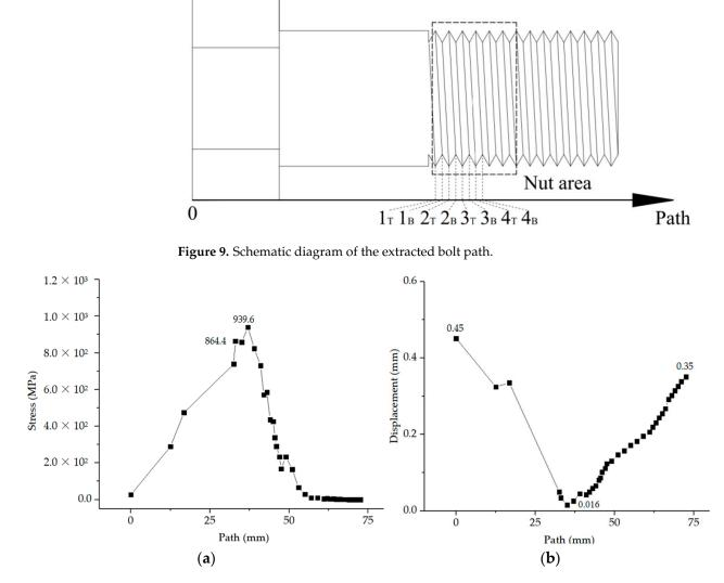
**Figure 10.** Stress and Displacement Line Chart along Bolt Path under Different Loads: (**a**) Fracture line diagram of UDHSB path stress under seismic load; (**b**) Line diagram of path displacement of UDHSB under seismic load.
