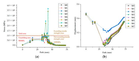
**Figure 12.** Distribution of stress S and displacement U of cracked bolt along path: (**a**) Path stress distribution of cracked bolt under seismic load; (**b**) Path displacement distribution of cracked bolt under seismic load.
