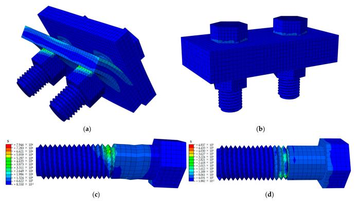
**Figure 8.** Bolt Stress Results: (**a**) Model stress nephogram under linear load; (**b**) Model displacement nephogram under seismic load; (**c**) Stress simulation diagram of UDHSB under linear load; (**d**) Stress simulation diagram of UDHSB under seismic load.
