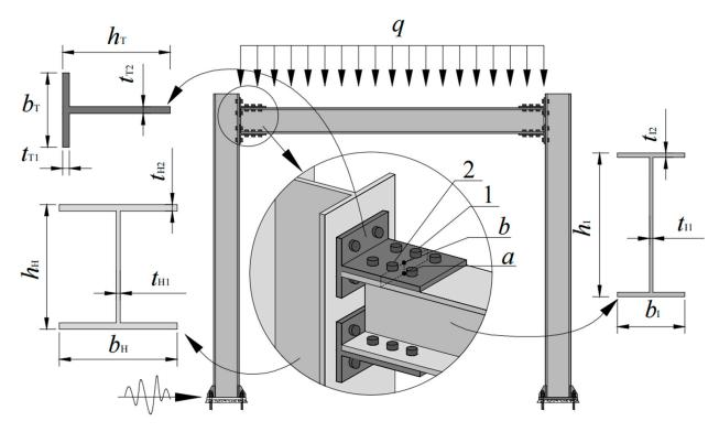
Figure 5. Seismic load application diagram of frame model.
