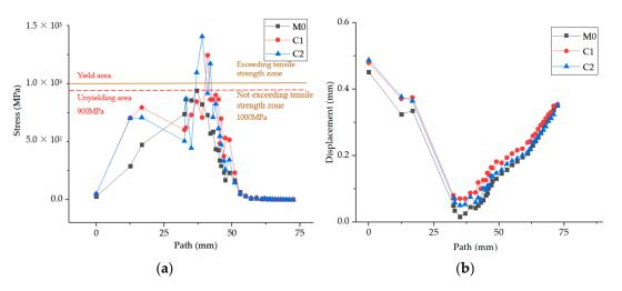
**Figure 15.** Distribution of stress S and displacement U along the path of thread tooth deformed bolt: (a) Stress distribution diagram of C1 and C2 along the path under seismic load; (b) Displacement distribution diagram of C1 and C2 along the path under seismic load.
