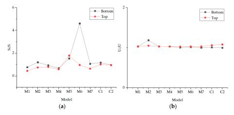
**Figure 17.** Comparison of stress and displacement between DHSB and UDHSB: (**a**) Stress multiple comparison diagram; (**b**) Displacement multiple comparison diagram.
