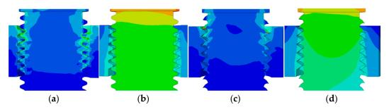
**Figure 14.** The bolt simulation stress S and displacement U of thread tooth deformation. (**a**) C1-S; (**b**) C1-U; (**c**) C2-S; (**d**) C2-U.
