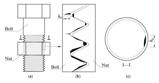
**Figure 1.** Schematic Diagram of Thread Damage: (**a**) Bolt and nut; (**b**) Thread tooth damage amplification diagram; (**c**) I-I cross-section.
