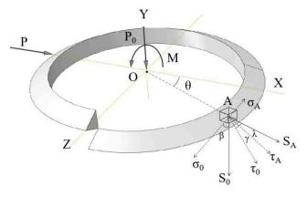
Figure 3. Specific force diagram of thread surface of bolt under transverse vibration load.
