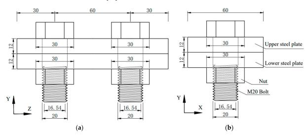
**Figure 4.** Schematic Diagram of Design Model: (**a**) Front view of design model; (**b**) Side view of design model.
