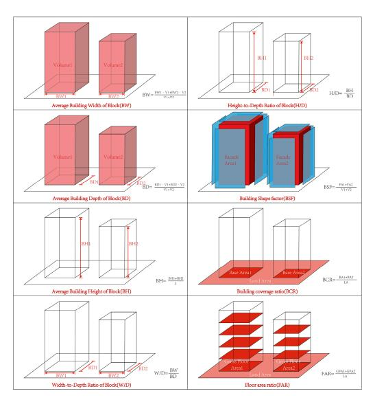
Figure 6. Calculation equation of block morphological parameters.
