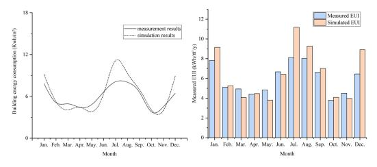
Figure 10. Comparison of measured and simulated EUI.
