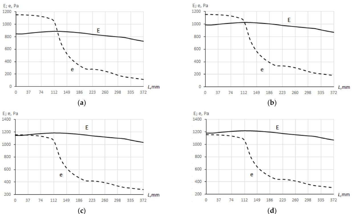
**Figure 11.** Graphs of changes in the partial pressure of water vapor  $e$  and partial pressure of saturated water vapor  $E$  in the area of metal structures that are not in contact with the attic air at a relative humidity in the attic of 70% and its temperature: (a)  $-15$  °C; (b)  $-10$  °C; (c)  $-5$  °C; and (d)  $-4$  °C.
