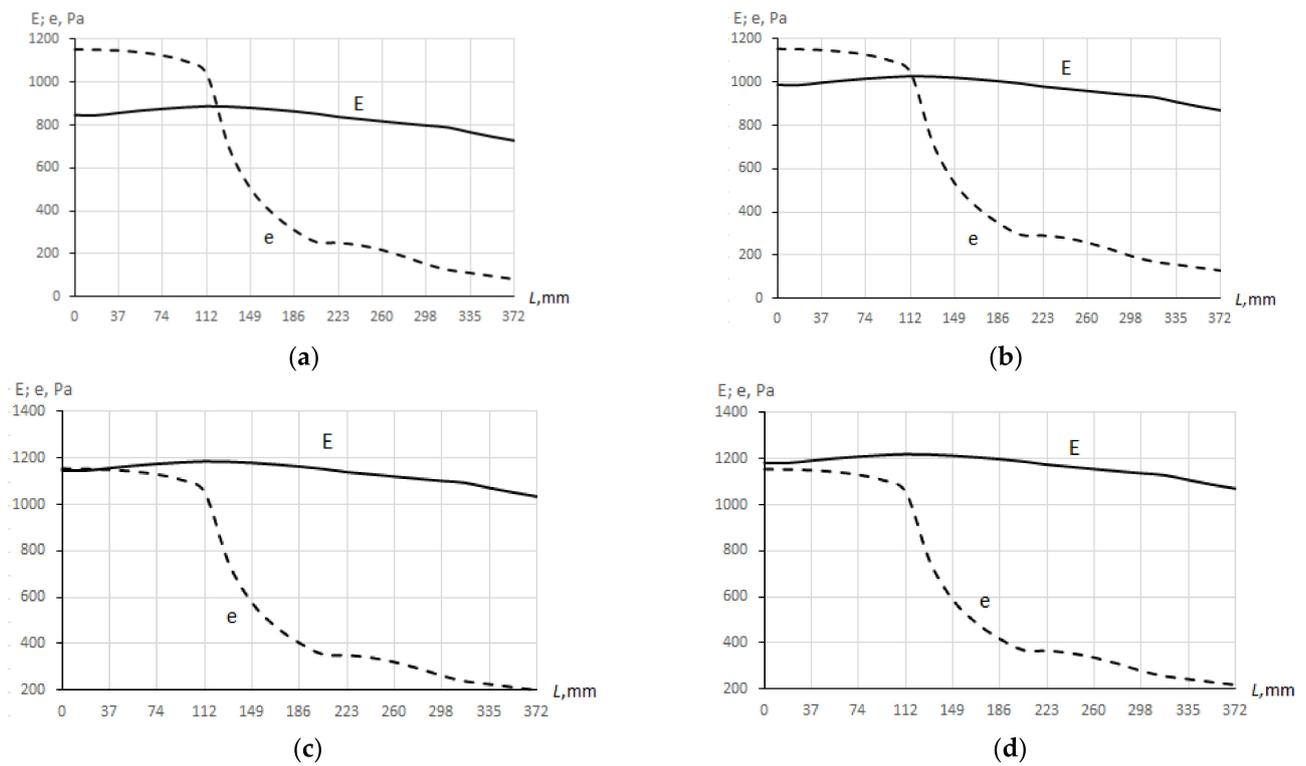
**Figure 12.** Graphs of changes in the partial pressure of water vapor  $e$  and partial pressure of saturated water vapor  $E$  in the area of metal structures that are not in contact with the attic air at a relative humidity in the attic of 50% and its temperature: (a)  $-15\text{ }^{\circ}\text{C}$ ; (b)  $-10\text{ }^{\circ}\text{C}$ ; (c)  $-5\text{ }^{\circ}\text{C}$ ; and (d)  $-4\text{ }^{\circ}\text{C}$ .
