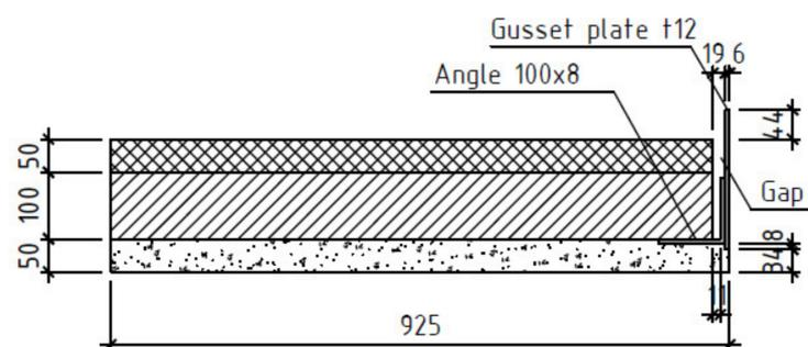
**Figure 15.** Calculation scheme with a gusset plate. The gaps between the angles and precast reinforced concrete elements are not filled with thermal insulation (units: mm).
