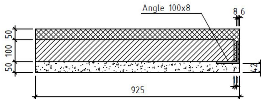
**Figure 18.** Calculation scheme without a gusset plate. The gaps between the angles and precast reinforced concrete elements are filled with thermal insulation (units: mm).
