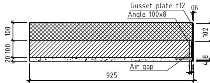
**Figure 20.** Calculation scheme with a gusset plate (units: mm). Thermal insulation—mineral wool with a density of  $200 \text{ kg/m}^3$  and a thickness of 100 mm.
