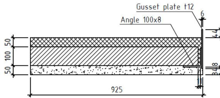
**Figure 8.** Calculation scheme with a gusset plate. The gaps between the angles and precast reinforced concrete elements are filled with thermal insulation (units: mm).
