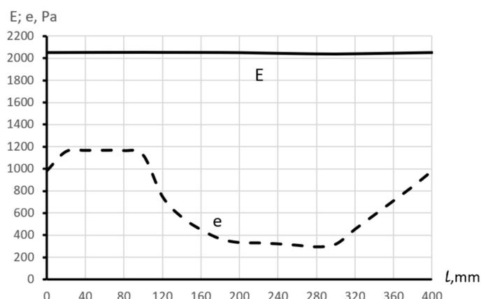
**Figure 23.** Graphs of changes in the partial pressure of water vapor  $e$  and partial pressure of saturated water vapor  $E$  in the area of metal structures that are not in contact with the attic air for calculation scheme without a gusset plate (thermal insulation—mineral wool with a density of  $200 \text{ kg/m}^3$  and a thickness of  $100 \text{ mm}$ ).
