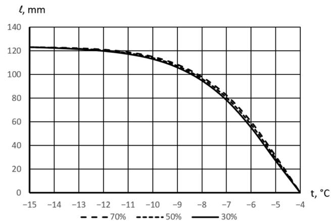
**Figure 14.** Graphs of the length of the condensation area along the perimeter of the section of the bottom chord of the truss depending on the temperature and relative humidity of the air in the attic.
