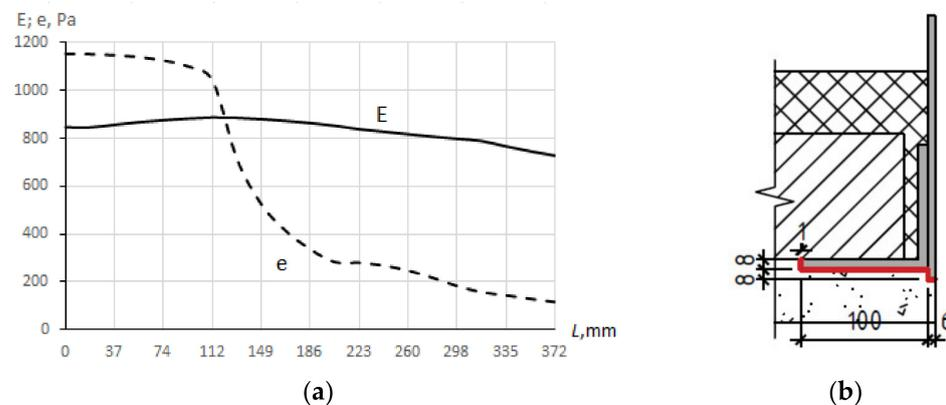
**Figure 10.** Graphs of changes in partial pressure of water vapor  $e$  and partial pressure of saturated water vapor  $E$  in the area of metal structures that do not come into contact with the attic air (a); the condensation area along the perimeter of the section of the bottom chord of the truss (units: mm) (b).
