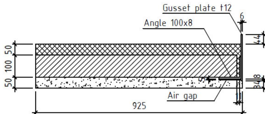
**Figure 16.** Calculation scheme with a gusset plate. Detachment of the finishing layer from the elements of the bottom chord of the truss (units: mm).
