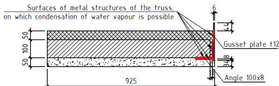
**Figure 7.** Surfaces of the metal elements of the truss's bottom chord, where condensation of water vapor is possible (units: mm).
