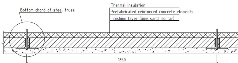
Figure 6. Construction of the existing attic ceiling (unit: mm).
