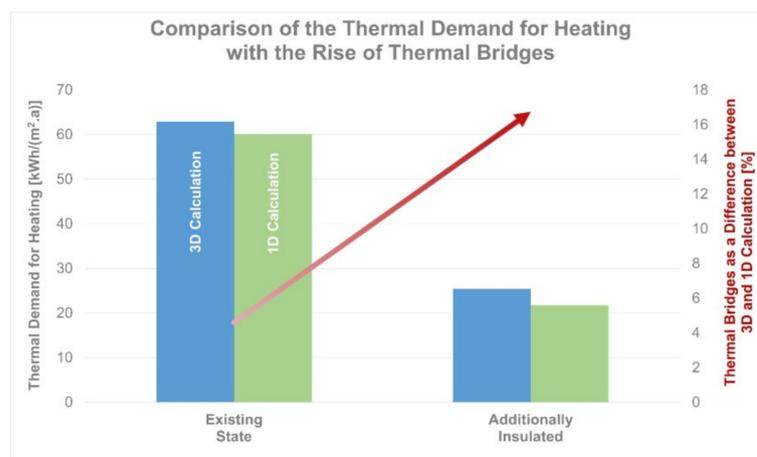
**Figure 1.** Comparison of heating demand with the increase in thermal bridges (Adapted from Ref. [2]). The proportion of thermal bridges is defined as the difference between 3D and 1D calculation of the heating demand. The calculations were performed for the existing, non-insulated facade and retrofitted (i.e., additionally insulated facade of an apartment building).
