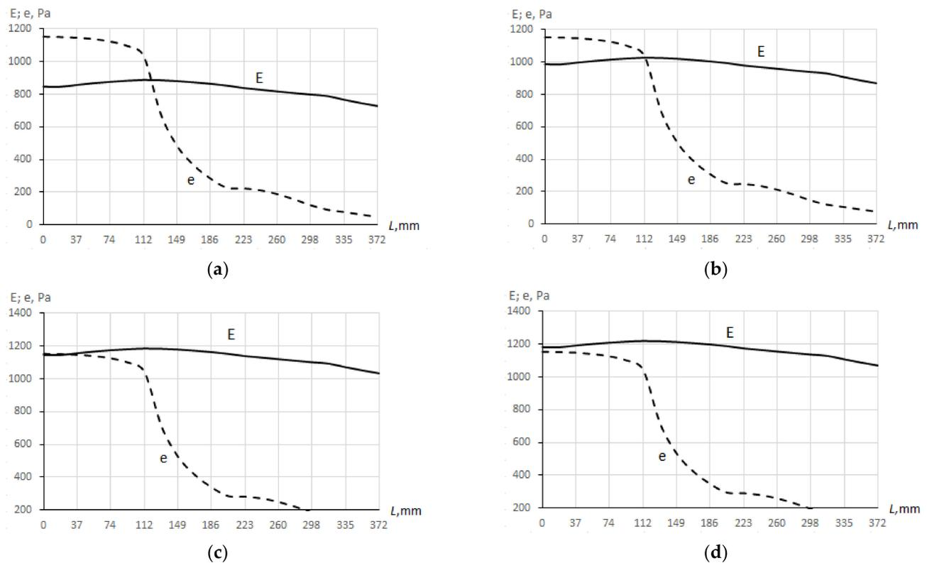
**Figure 13.** Graphs of changes in the partial pressure of water vapor  $e$  and partial pressure of saturated water vapor  $E$  in the area of metal structures that are not in contact with the attic air at a relative humidity in the attic of 30% and its temperature: (a)  $-15\text{ }^{\circ}\text{C}$ ; (b)  $-10\text{ }^{\circ}\text{C}$ ; (c)  $-5\text{ }^{\circ}\text{C}$ ; and (d)  $-4\text{ }^{\circ}\text{C}$ .
