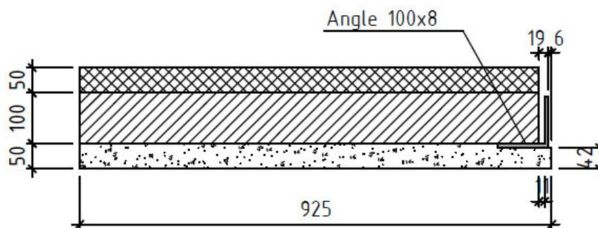
**Figure 19.** Calculation scheme without a gusset plate. The gaps between the angles and precast reinforced concrete elements are not filled with thermal insulation (units: mm).
