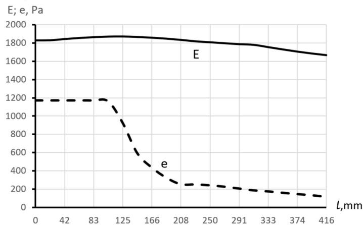
**Figure 21.** Graphs of changes in the partial pressure of water vapor  $e$  and partial pressure of saturated water vapor  $E$  in the area of metal structures that are not in contact with the attic air for calculation scheme with a gusset plate (thermal insulation—mineral wool with a density of  $200 \text{ kg/m}^3$  and a thickness of 100 mm).
