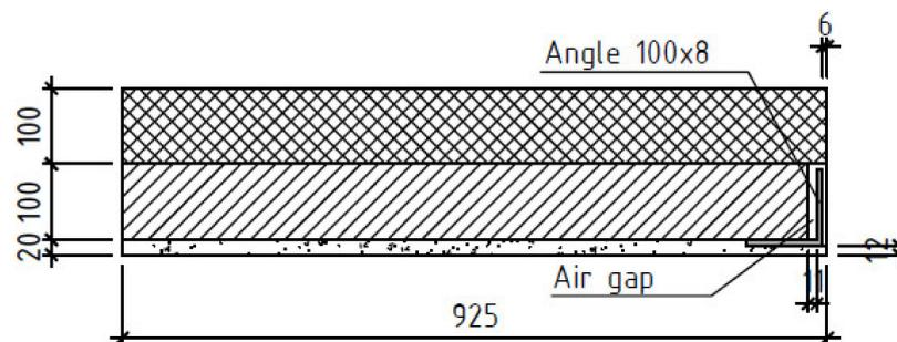
**Figure 22.** Calculation scheme without a gusset plate (units: mm). Thermal insulation—mineral wool with a density of  $200 \text{ kg/m}^3$  and a thickness of 100 mm.
