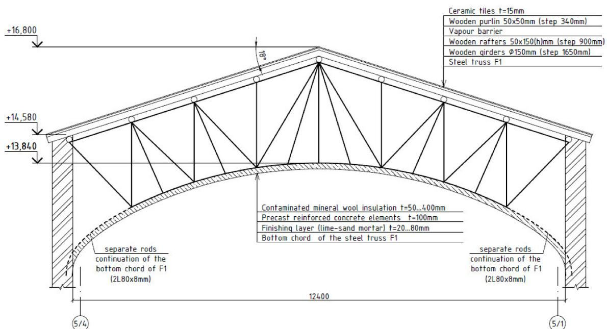
Figure 3. Schematic drawing of the truss.
