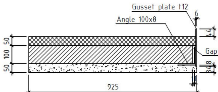
**Figure 17.** Calculation scheme with a gusset plate. Partial filling of the gap with thermal insulation between precast concrete elements and metal structures (units: mm).
