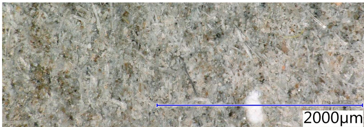
Figure 4. Detail of used fiber cement board, tensile failure.
