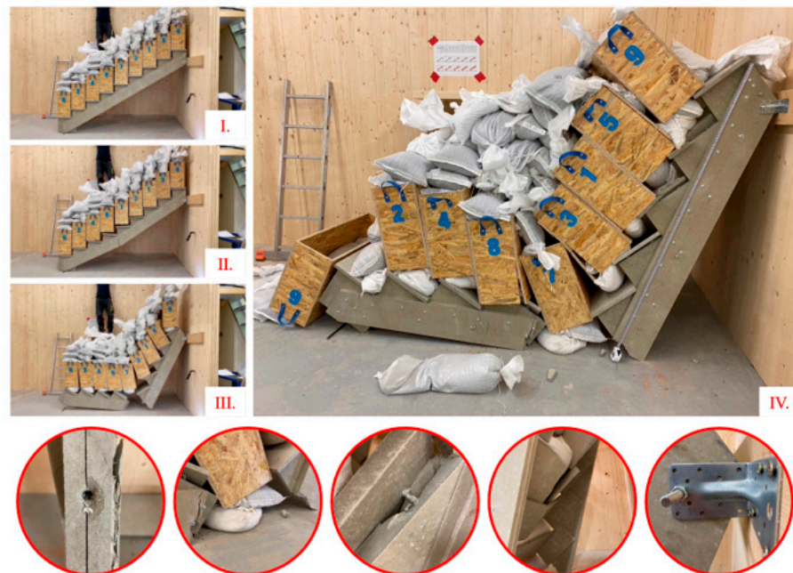
Figure 17. Failed interior staircase structure made from cement fiber boards under loading of 9.26 \text{ kN/m}^2 , detailed photo documentation of failed structure. Where (I) is the structure of the staircase before the crack appeared, (II) the first appearance of a crack on the structure, (III) broken staircase structure, (IV) detailed view of the broken structure.
