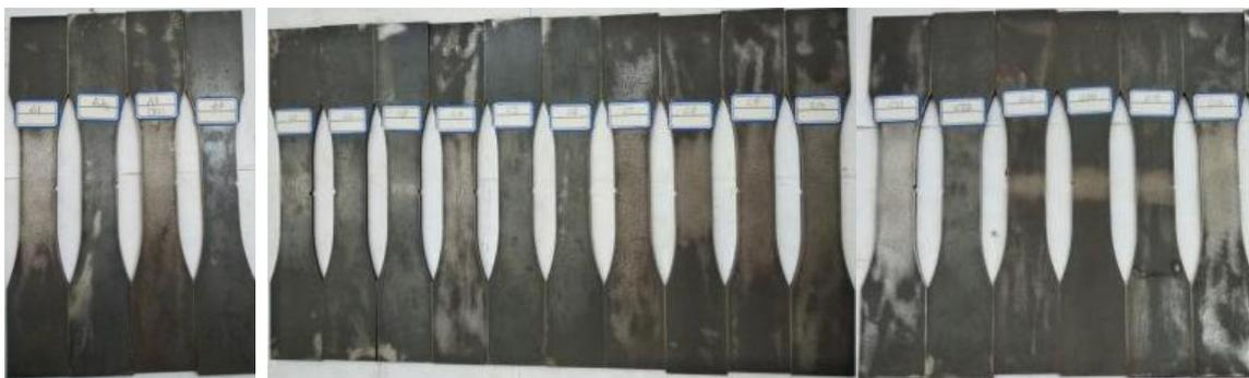
Figure 2. Pictures of the Q460C steel notched plates.
