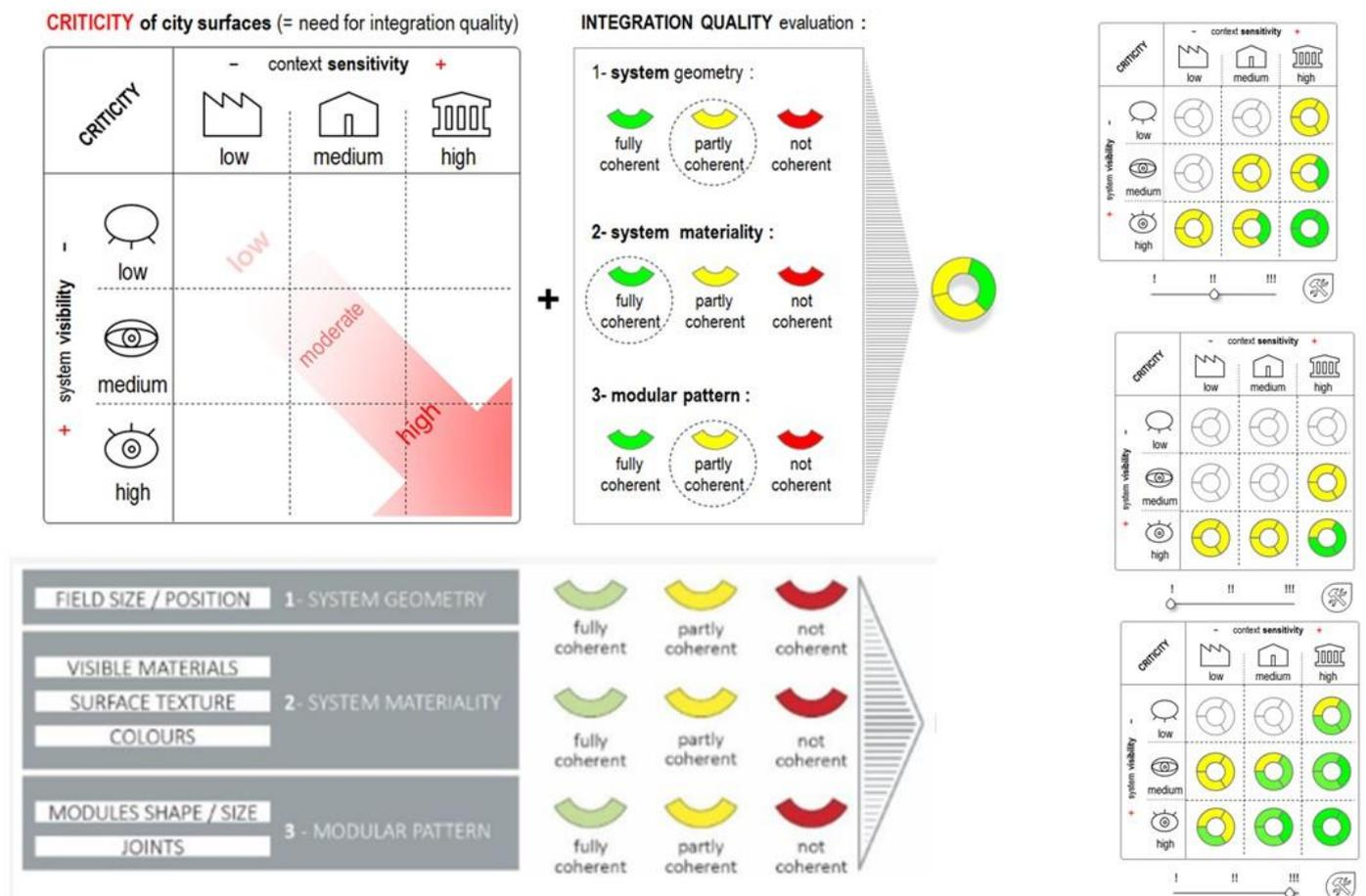
**Figure 5.** “Criticity map” considering visibility and sensitivity (Source: Authors’ elaboration from LESO-QSV—Architectural integration tool, [https://www.epfl.ch/labs/leso/research/domains/renewables\\_integration/leso-qsv](https://www.epfl.ch/labs/leso/research/domains/renewables_integration/leso-qsv), accessed on 14 February 2023).
