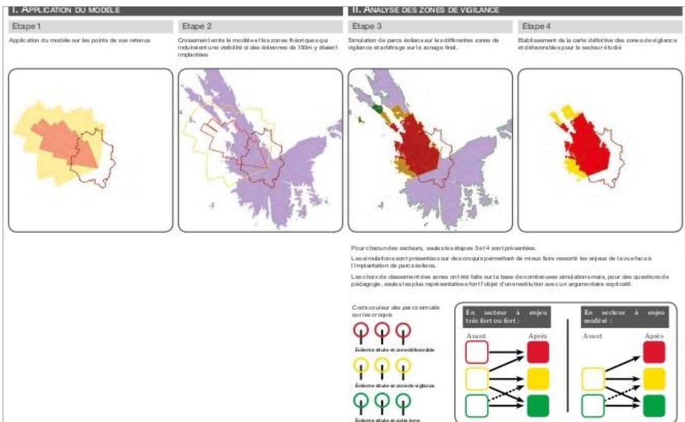
**Figure 15.** Zoning of wind turbines in the Vézelay landscape (France) based on angle of view and distance of the turbines: unfavorable (red), caution (yellow), and other zones (green) (Source: [84]).
