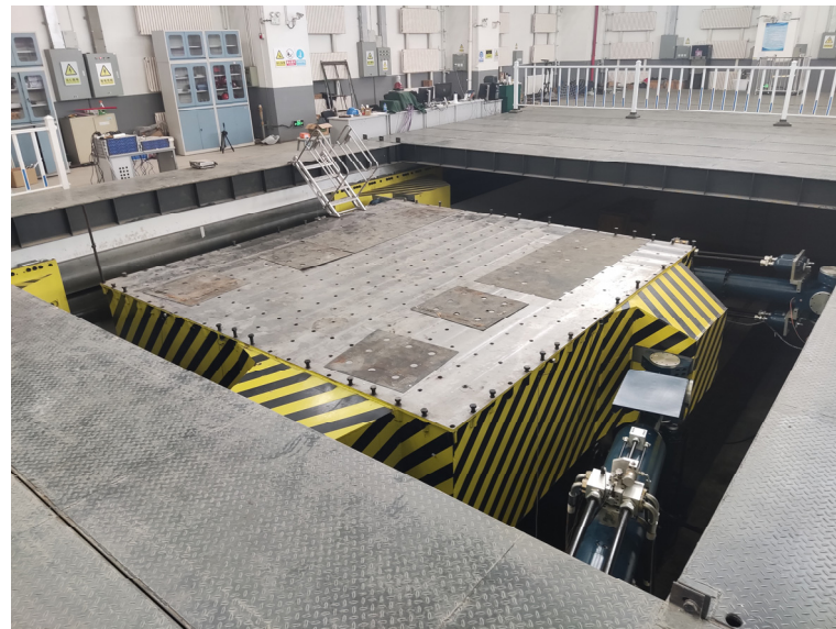
Figure 7. The large-scale multi-functional shaking table array at Beijing University of Civil Engineering and Architecture.
