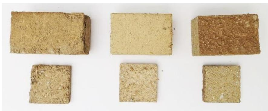
**Figure 34.** The appearance of hardened mixtures (halves of  $4 \times 4 \times 16$  cm beams) on the surface and in the cross section, E—left, EL—middle, ELC—right.
