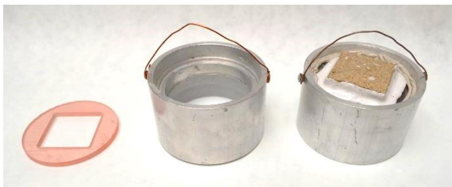
**Figure 35.** Arrangement of the water vapour permeability test.
