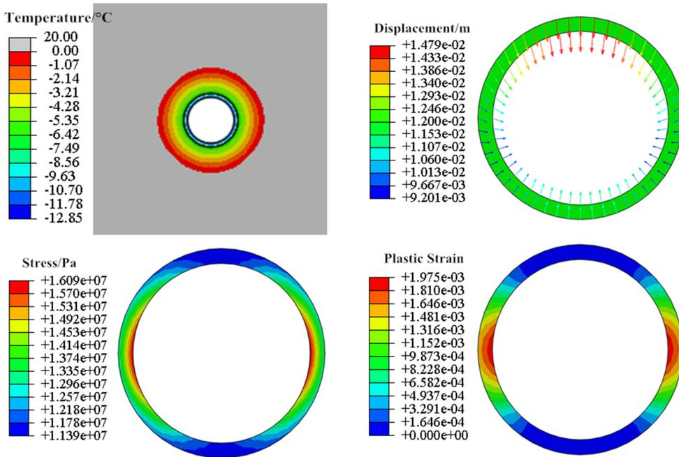
(b) Stress and plastic strain with a porosity of 0.23
