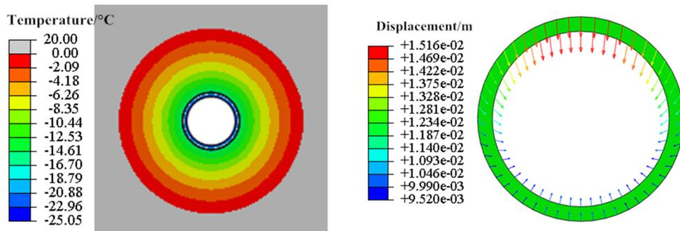
(c) Calculation results for a temperature difference of 50 °C
