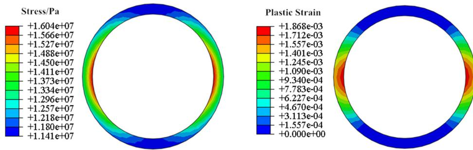
(a) Calculation results for a temperature difference of 30 °C
