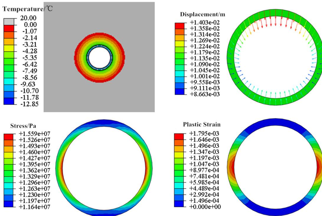
(a) Stress and plastic strain at the thermal expansion coefficient of  $3 \times 10^{-6} / ^\circ\text{C}$
