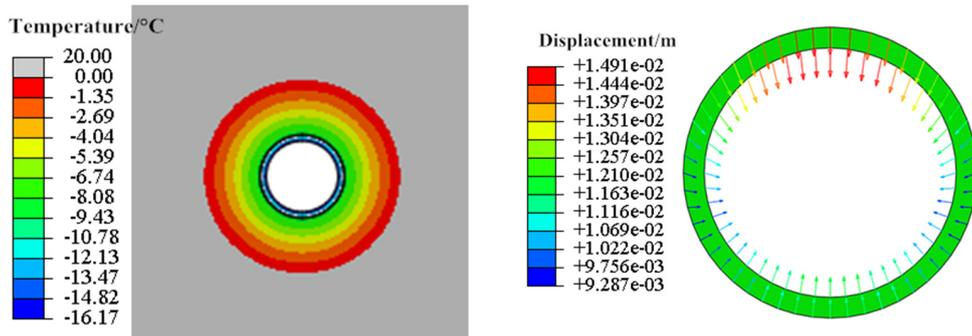
(b) Calculation results for a temperature difference of 40 °C
