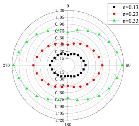
**Figure 9.** Annular distribution of the frost heave force of rock mass with different water content.
