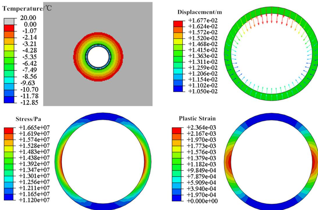
(c) Stress and plastic strain at the thermal expansion coefficient of  $7 \times 10^{-6}/^{\circ}\text{C}$
