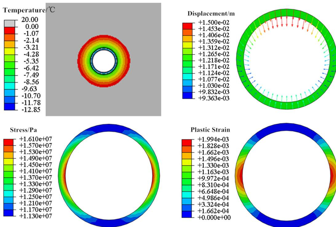
(b) Stress and plastic strain at the thermal expansion coefficient of  $5 \times 10^{-6}/^{\circ}\text{C}$
