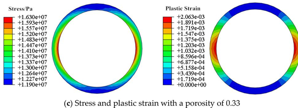
Figure 10. Effect of different porosity on bearing characteristics.
