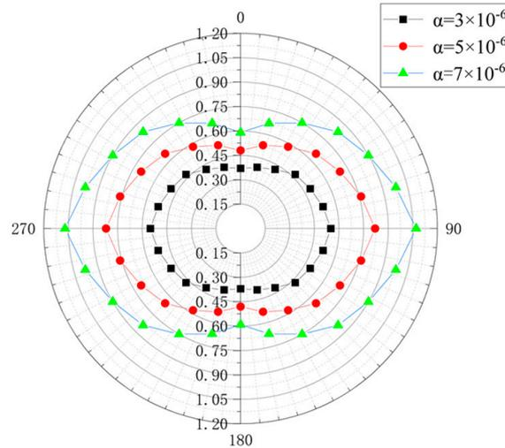
Figure 5. Annular distribution of frost heave force of rock mass with different thermal expansion coefficients (unit: MPa).
