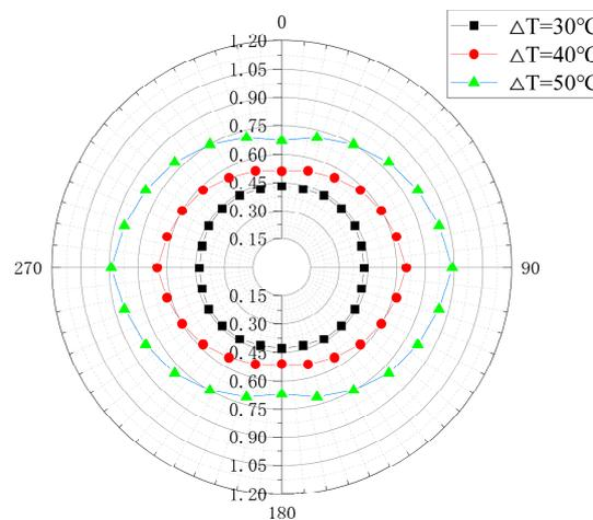
Figure 7. Annular distribution of frost heave force of rock mass with different temperature differences.
