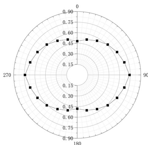
**Figure 3.** Annular distribution of frost heave force of rock mass (unit: MPa).
