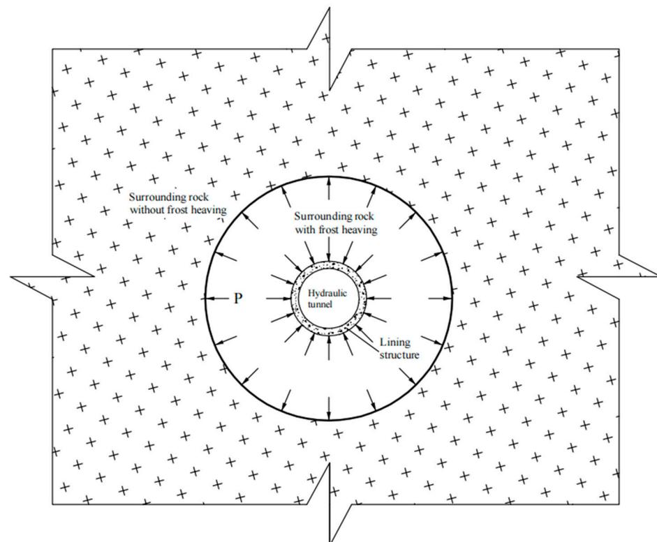
**Figure 1.** Schematic diagram of lining structure under frost expansion force.
