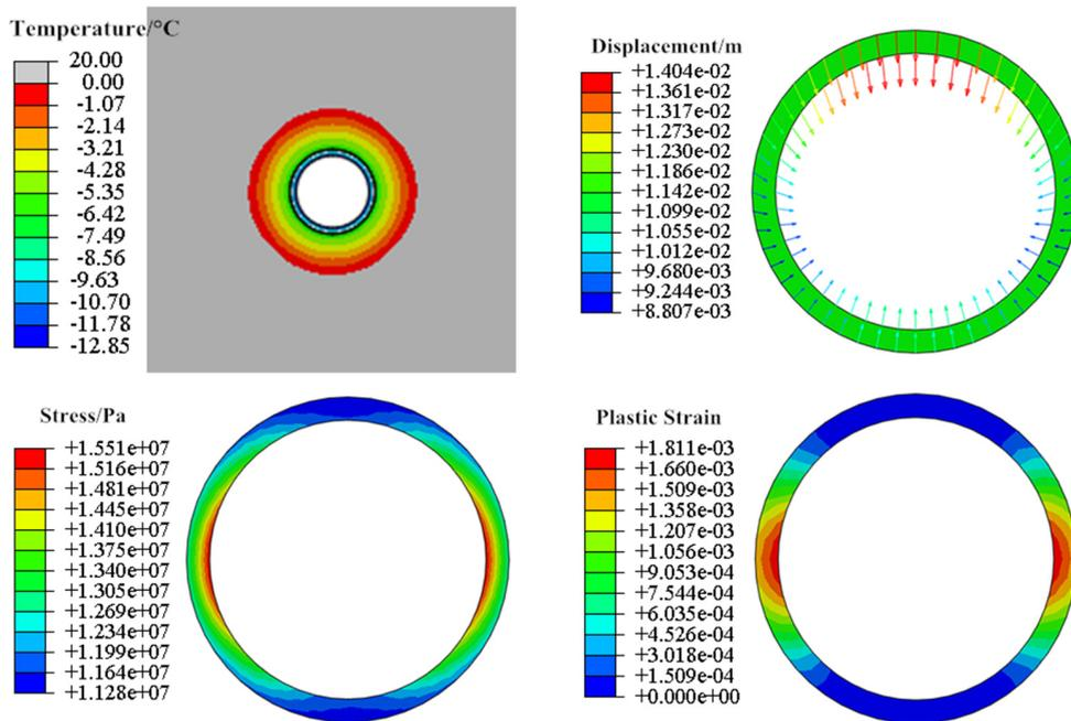
(a) Stress and plastic strain with a porosity of 0.13
