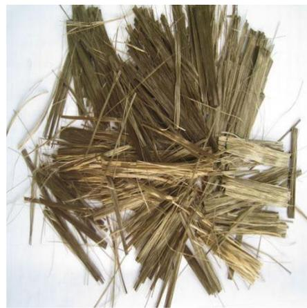
**Figure 4.** Basalt fibers.
