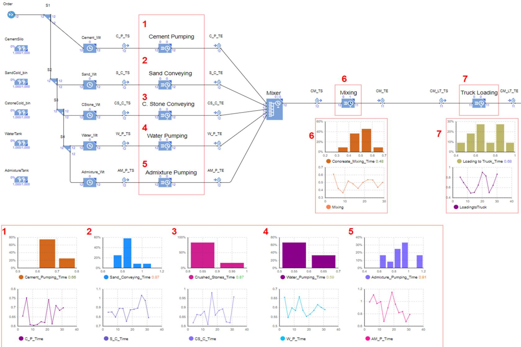
Figure 15. Digital Twin Operational Model.
