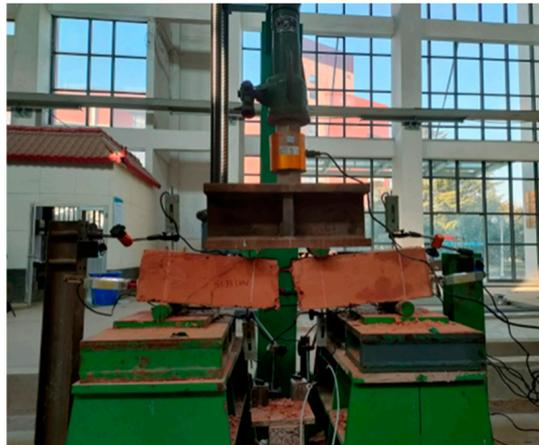
**Figure 7.** Splitting-pull-out failure (specimen GC40-16-7d-H).
