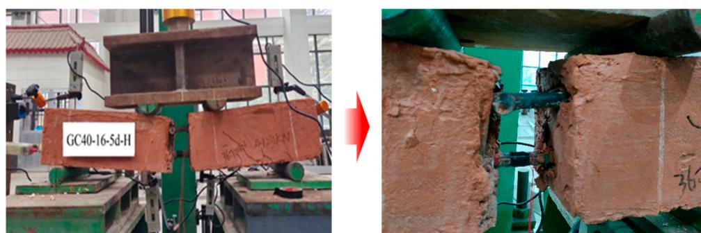
**Figure 5.** Steel bar pull-out failure (specimen GC40-16-5d-H).
