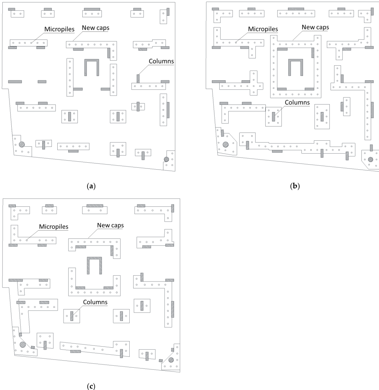
Figure 6. Layouts of the three proposed micropile configurations: (a) first approach, (b) second approach, and (c) third approach.
