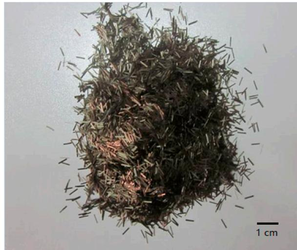
**Figure 1.** Basalt fiber.
