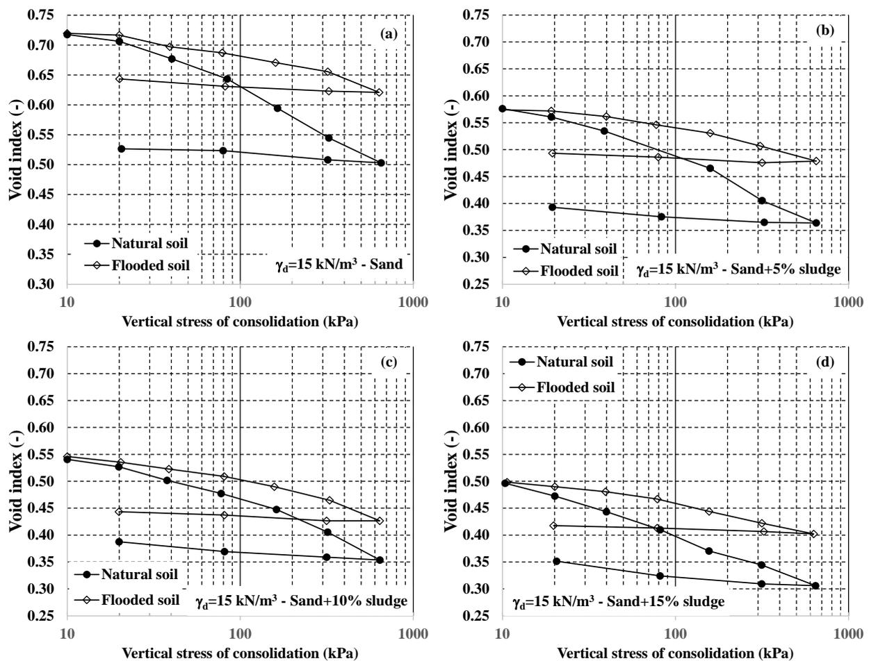
**Figure 13.** Variation of the void index with the vertical stress of consolidation obtained through double oedometer tests, for dry apparent specific weight of  $15.0 \text{ kN/m}^3$ : (a) sand, (b) sand plus 5% sewage sludge, (c) sand plus 10% sludge, (d) sand plus 15% sludge.
