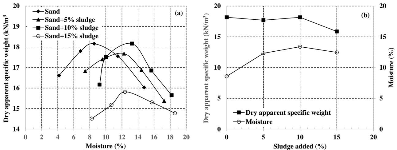
**Figure 5.** (a) Compaction curves of the tested materials and (b) Percent sludge versus maximum apparent dry specific weight and versus optimum moisture content.
