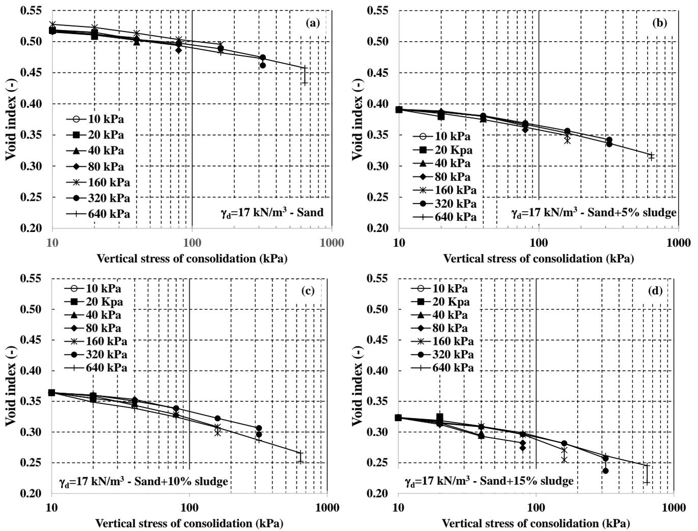
Figure 7. Variation of the void index with the vertical stress of consolidation obtained through single oedometer tests, for dry apparent specific weight of  $17.0 \text{ kN/m}^3$ : (a) sand, (b) sand plus 5% sewage sludge, (c) sand plus 10% sludge, (d) sand plus 15% sludge.
