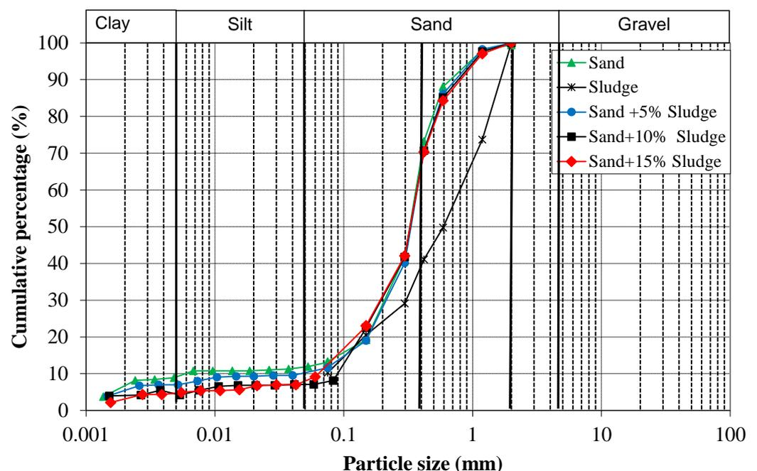
**Figure 4.** Particle soil distribution, sewage sludge, and different soil–sludge mixtures analyzed.
