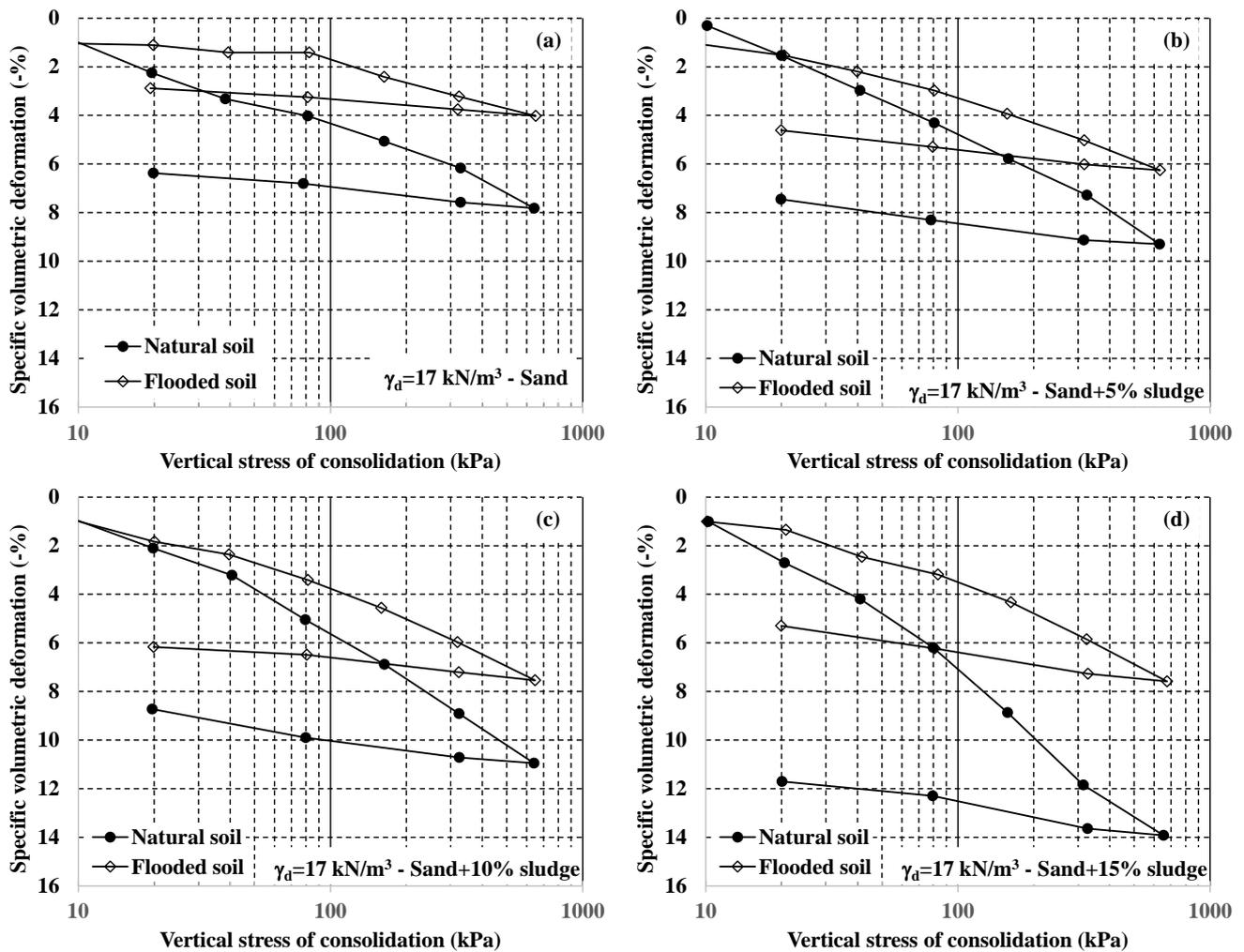
**Figure 16.** Variation of specific volumetric deformation with the vertical consolidation stress obtained through double oedometer tests, for dry apparent specific weight of  $17.0 \text{ kN/m}^3$ : (a) sand, (b) sand plus 5% sewage sludge, (c) sand plus 10% sludge, (d) sand plus 15% sludge.
