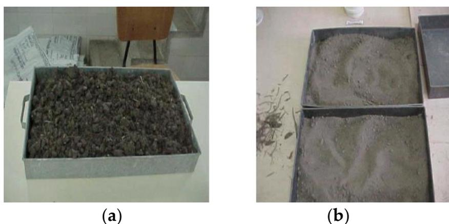
**Figure 1.** (a) Dry sludge and (b) sieved sludge obtained from a STP.
