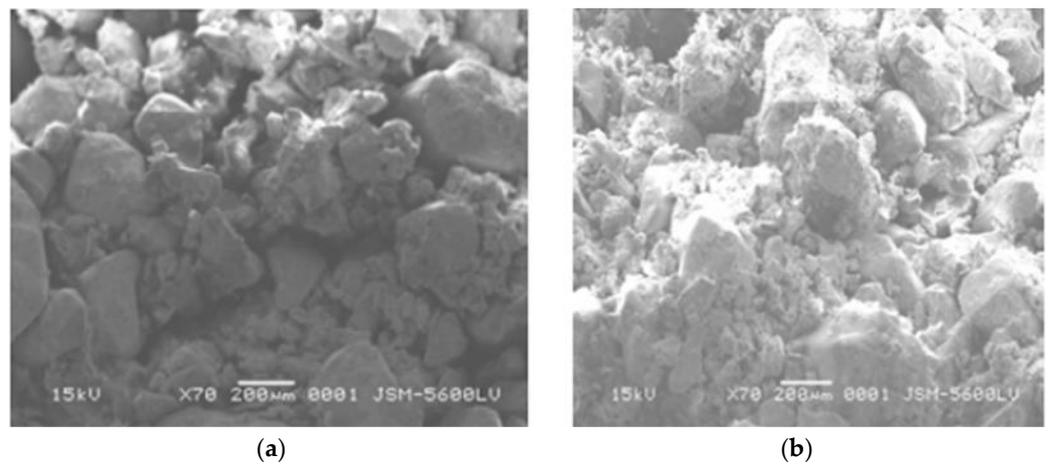
**Figure 12.** Electron microscopy of (a) natural soil—packaging, and (b) soil-sludge mixture—Quartz grains bonded with silts, clays, and soil-sludge organic matter.
