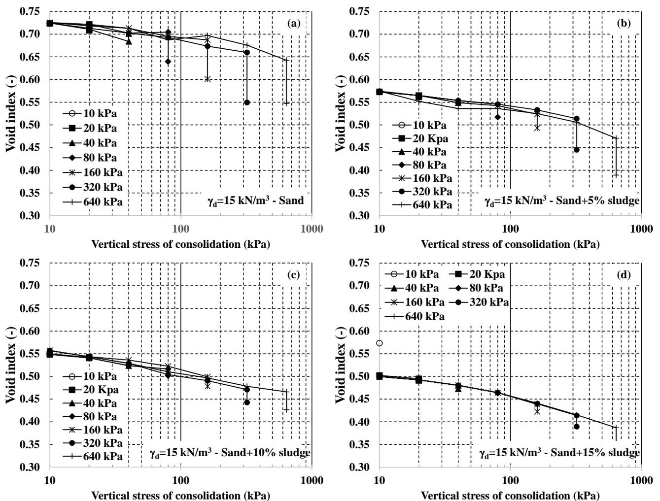
**Figure 6.** Variation of the void index with the vertical stress of consolidation obtained through single oedometer tests, for dry apparent specific weight of  $15.0 \text{ kN/m}^3$ : (a) sand, (b) sand plus 5% sewage sludge, (c) sand plus 10% sludge, (d) sand plus 15% sludge.
