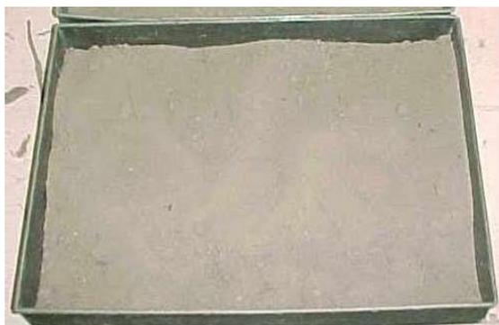
**Figure 2.** Natural soil—Silt sand.
