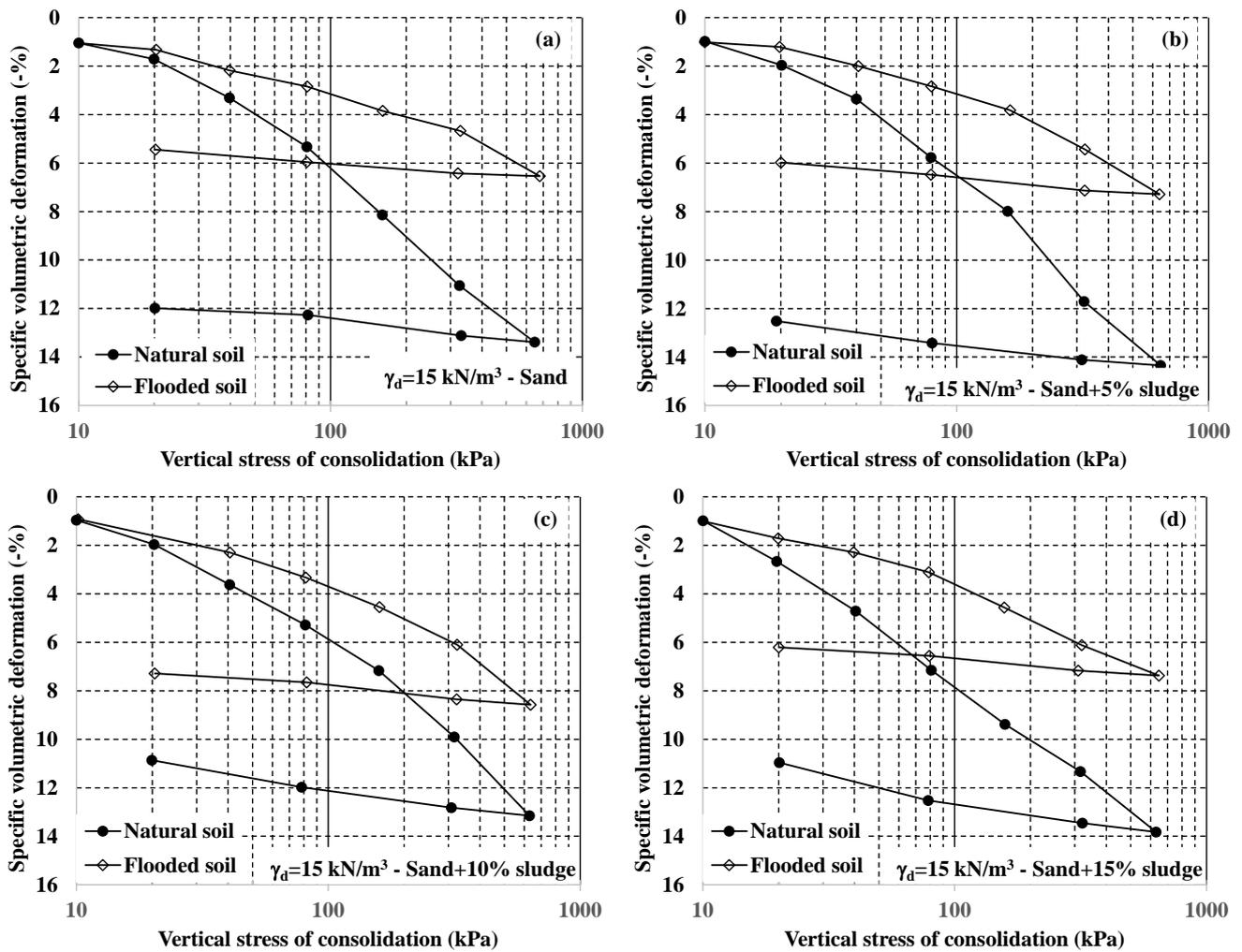
**Figure 14.** Variation of the void index with the vertical stress of consolidation obtained through double oedometer tests, for dry apparent specific weight of  $17.0 \text{ kN/m}^3$ : (a) sand, (b) sand plus 5% sewage sludge, (c) sand plus 10% sludge, (d) sand plus 15% sludge.
