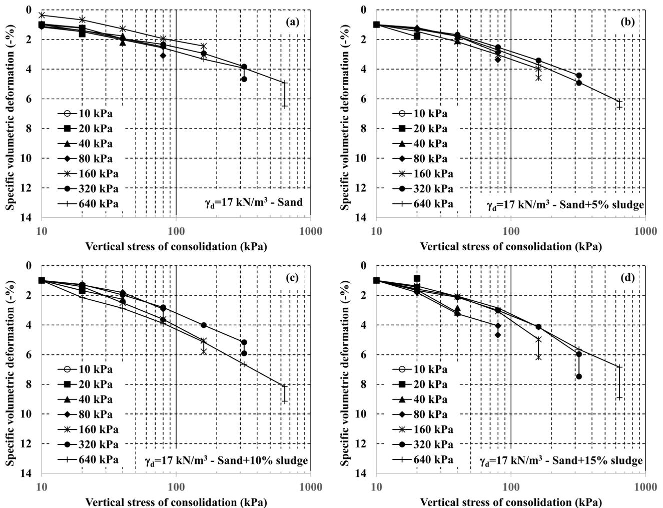
Figure 9. Variation of specific volumetric deformation with the vertical consolidation stress obtained through single oedometer tests, for dry apparent specific weight of  $17.0 \text{ kN/m}^3$ : (a) sand, (b) sand plus 5% sewage sludge, (c) sand plus 10% sludge, (d) sand plus 15% sludge.
