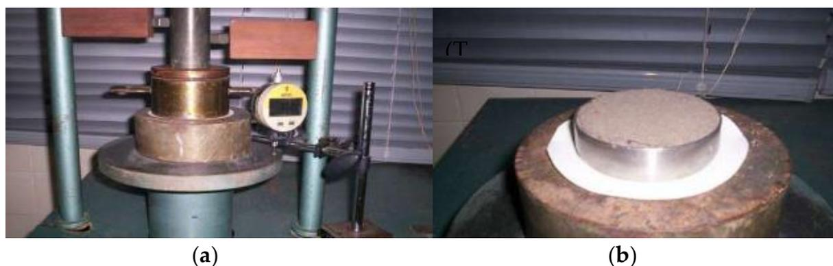
**Figure 3.** Compression mold at the beginning and after static compression: (a) Mold in the press at the start of compaction; (b) Mold after compaction.
