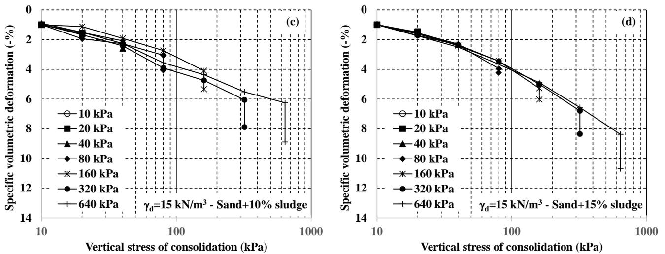
Figure 8. Variation of specific volumetric deformation with the vertical consolidation stress obtained through single oedometer tests, for dry apparent specific weight of  $15.0 \text{ kN/m}^3$ : (a) sand, (b) sand plus 5% sewage sludge, (c) sand plus 10% sludge, (d) sand plus 15% sludge.
