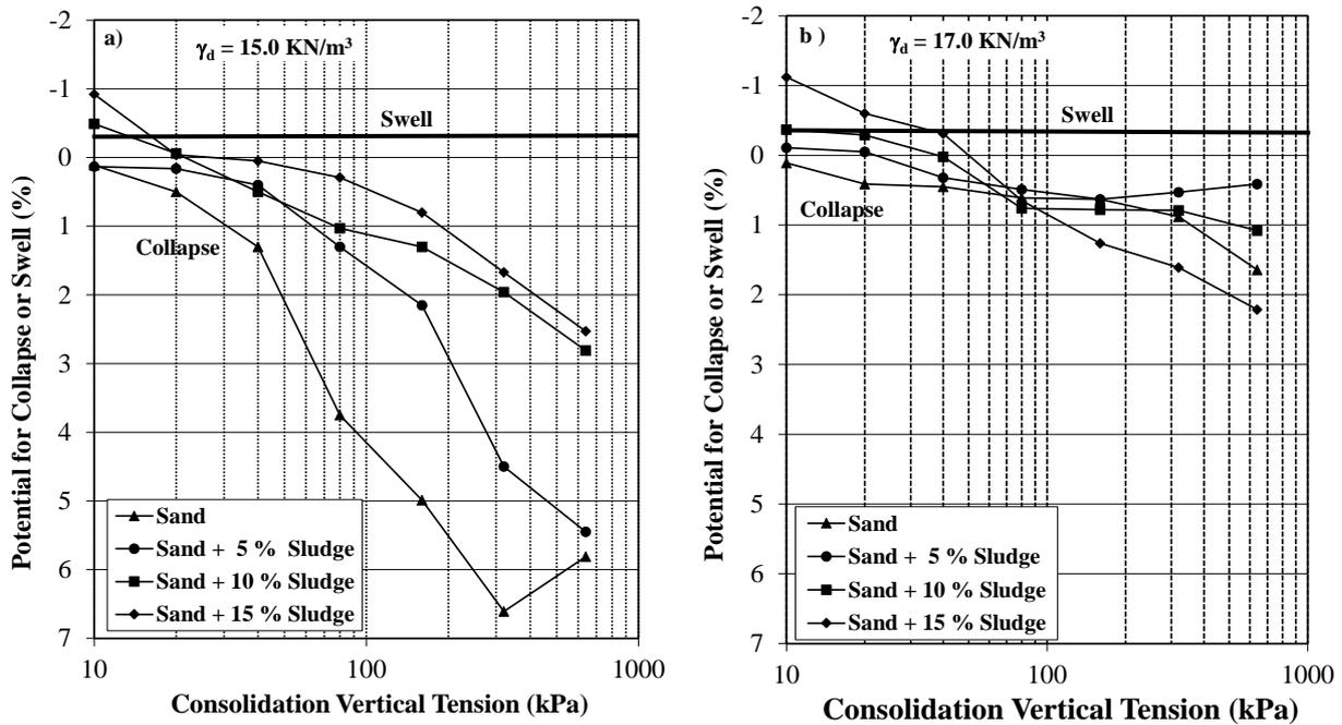
Figure 10. Variation of collapse or expansion potential values with vertical consolidation stress, (a) for  $\gamma_d = 15.0 \text{ kN/m}^3$  and (b) for  $\gamma_d = 17.0 \text{ kN/m}^3$ .
