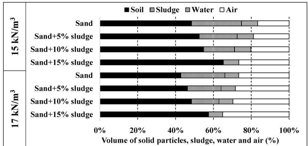
Figure 11. Volume, in %, of the different mixture components.
