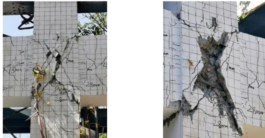
**Figure 14.** Crack development and failure of specimen ZJ-3.
