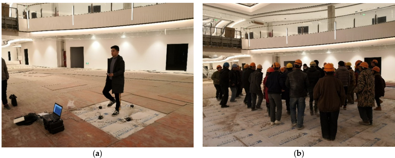
Figure 6. Field tests of human-induced vibration: (a) single pedestrian walking in place; (b) 40 pedestrians walking in place.
