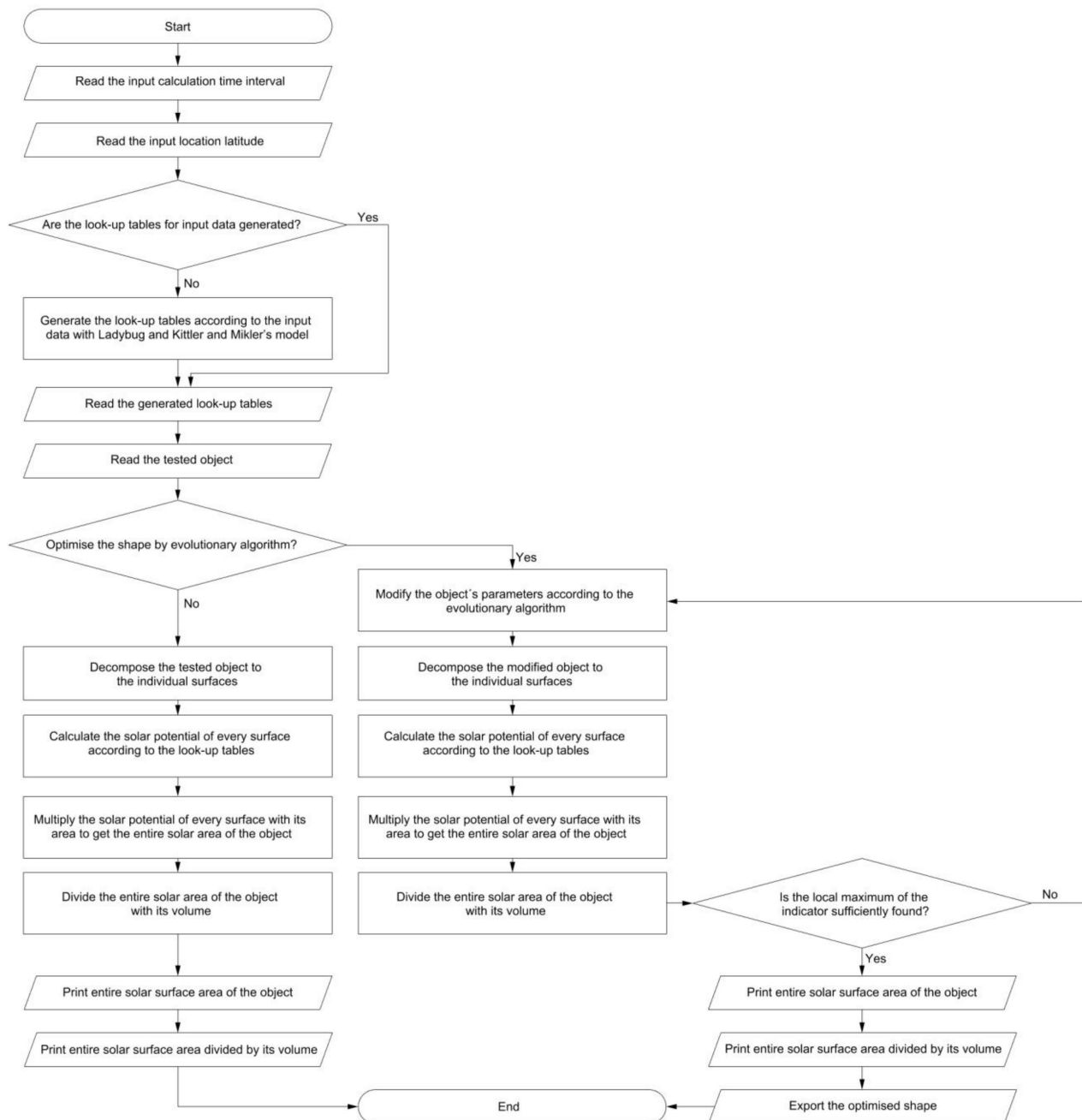
Figure 3. The algorithm for solar-surface-area-to-volume ratio. The algorithm without the evolutionary optimisation part was also scripted in Javascript to help the public calculate and visualise the solar surface area and solar-surface-area-to-volume ratio online.
