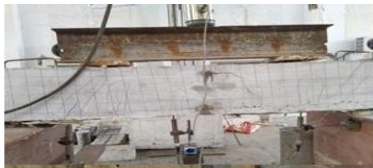
Figure 15. Crack pattern for Beam 2.
