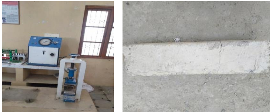
Figure 2. Flexural strength test.
