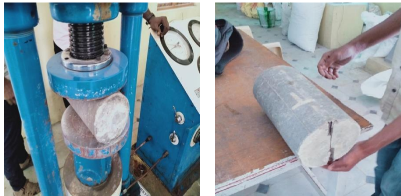
Figure 3. Split tensile strength test.
