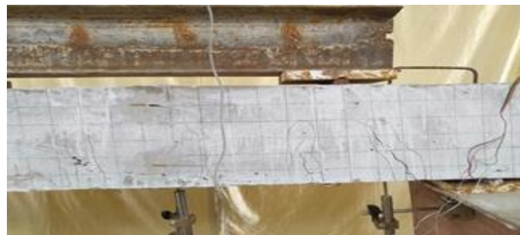
Figure 16. Crack pattern for Beam 3.
