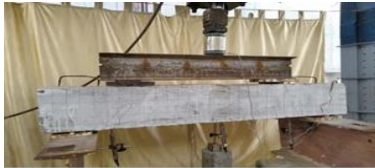
Figure 14. Crack pattern for Beam 1 (controlled concrete).
