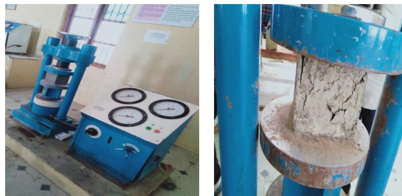
Figure 1. Compressive strength test.
