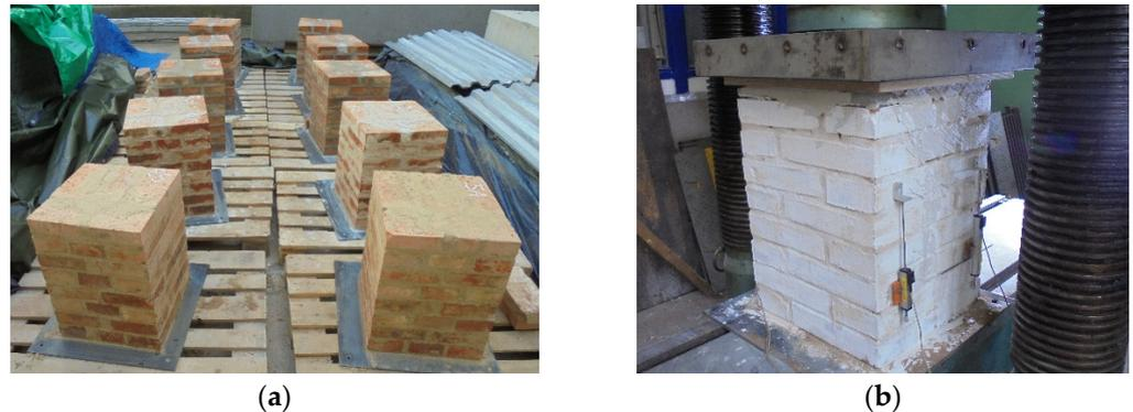
**Figure 5.** Pictures of the samples: (a) all 10 pillar samples; (b) sample 5A placed in a loading device during the experiments.
