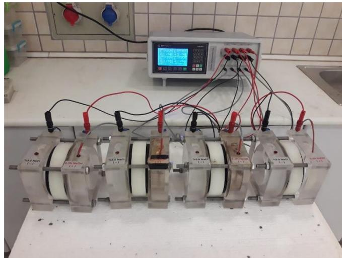
**Figure 3.** The RCPT test device.
